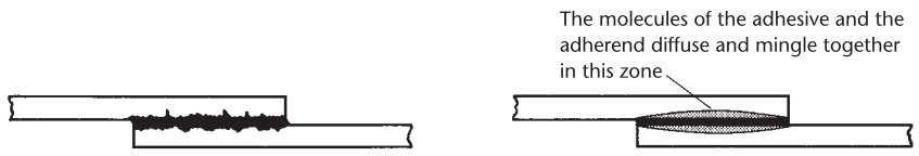
(a) Elements of the bonded joint
