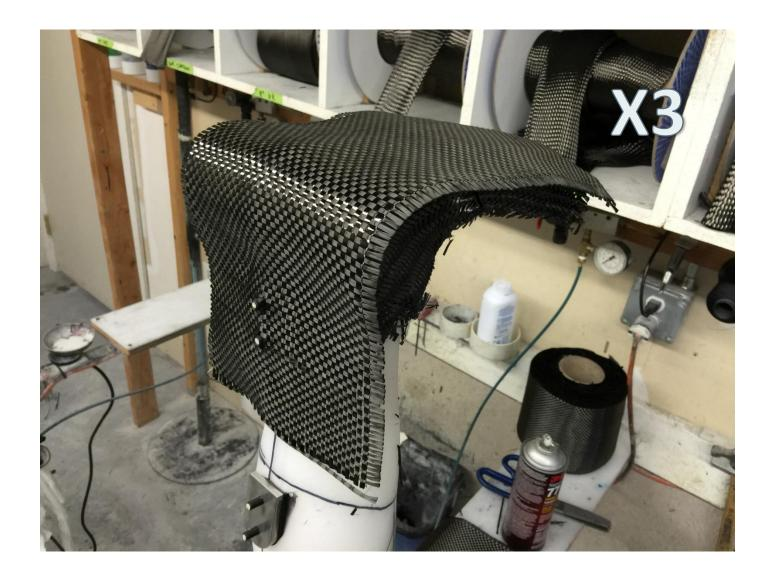
Cover footplate with 3ea layers CT6 12K carbon tape in 0/90 orientation.
