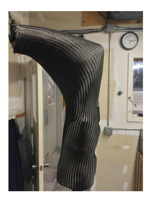
Split the final layer open by the ankle to get the fabric to lay down nicely.
