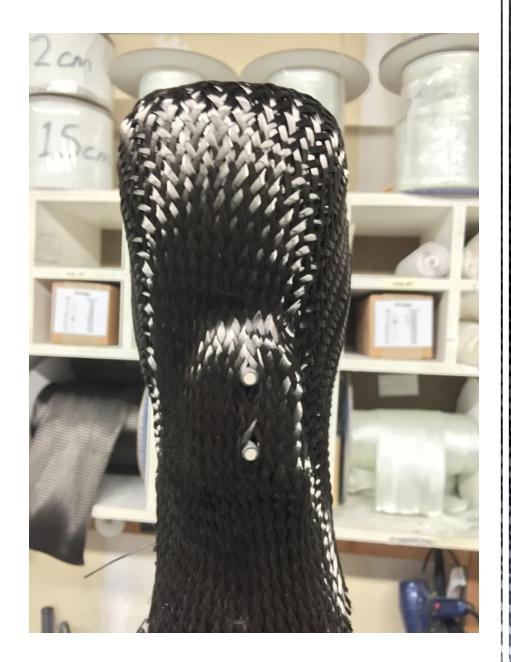
Place the lamination dummies on the model with the exposed set screws to hold it in position.
