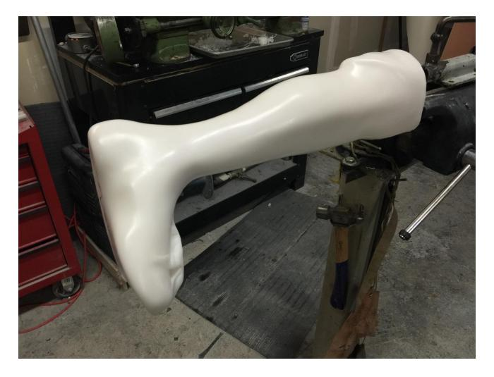
Using 1/8" thick polypropylene pull the entire model using the same technique you would use for a standard plastic AFO. Ensure there are no wrinkles or excessive stretch within the trim lines. This will serve as both a spacer for the plastic and foam liners as well as a releasable surface to laminate on.
