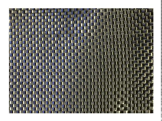
Standard 12k weight 45° degree carbon tubular braid.
