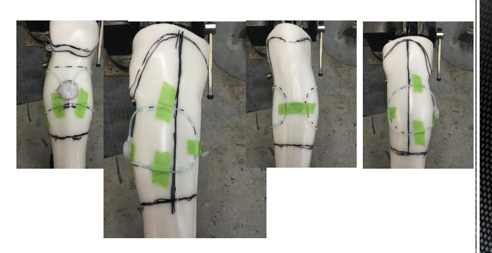
Tape Teflon™ tubing into position.
