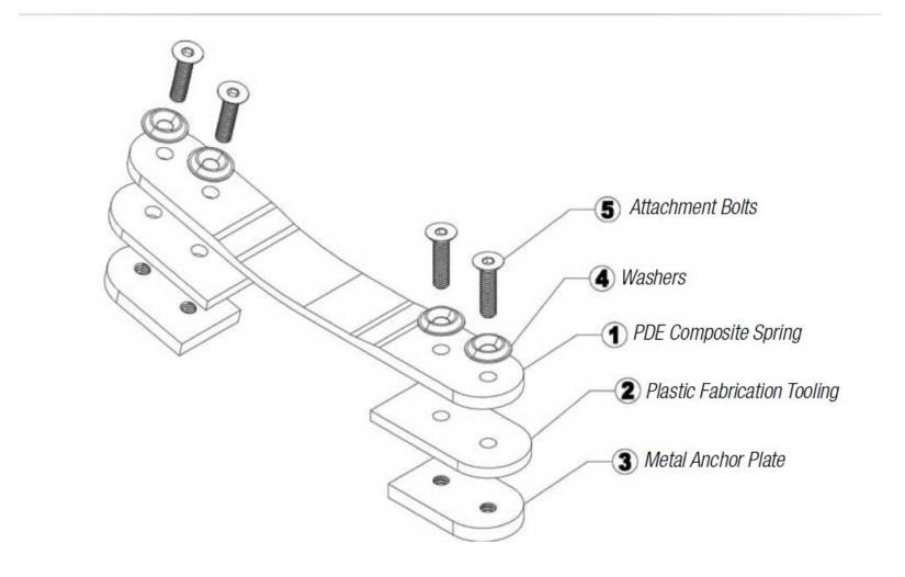
Assemble components in this configuration.
