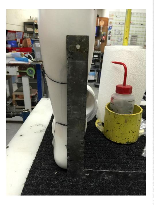
This reference mark is the ideal placement for the spring. In the event this mark is noticeably off center of the calf it is ok to alter it within a few degrees for aesthetics.
