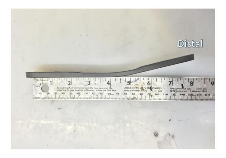
The PDE spring is not symmetrical. The bend is closer to the distal end of the spring. Shown here the distal location of the spring is to the right side.
