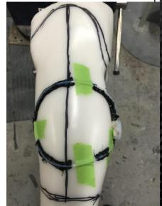
With the Teflon™ tubing in position using masking tape. Use Composite 1 adhesive to liberally glue down the exposed Teflon™.
