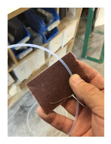
The easiest way to do this is by folding the sand paper and pulling the Teflon™ ™ through.
