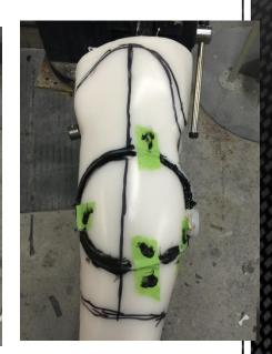
Wipe excess adhesive off of the routed tubing. The masking tape is a great place to wipe all excess that isn't needed.
