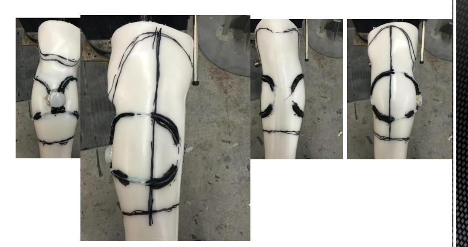
Once the Composite1 adhesive has cured remove the masking tape. Use additional Composite1 adhesive and bond the open areas.
