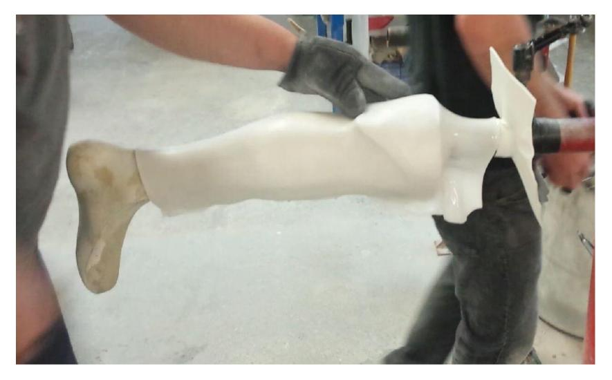
Using a 1/8" thick soft plastic interface material (Proflex™ with silicone) Pull the proximal posterior cuff. Be sure to make this section large enough to extend 1 ½" past midline join of anterior shell and posterior cuff. Label this piece with patient information and set aside for finishing.
