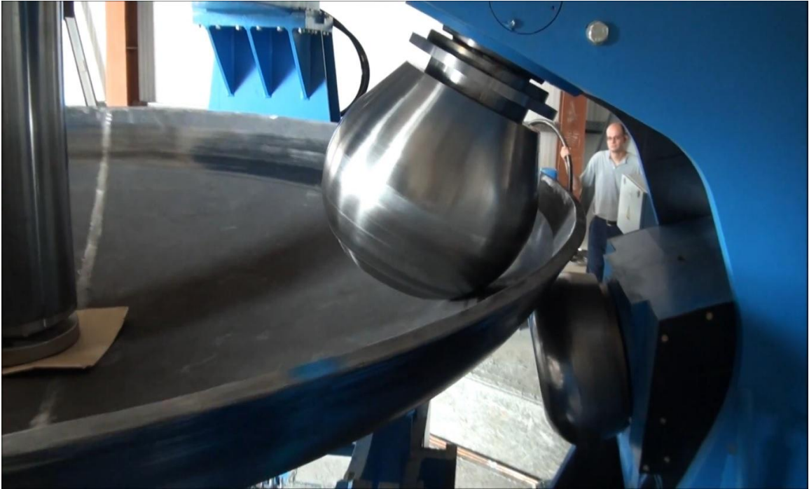
Figure 10.5 – Head Spinning (Flanging)
