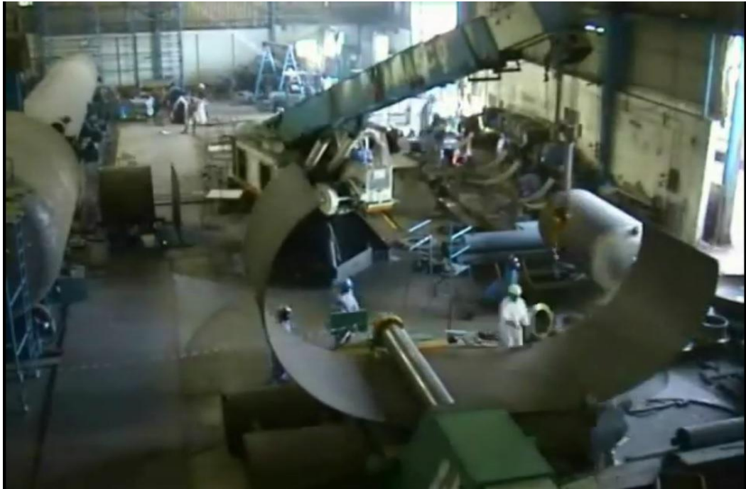
Figure 11.1 – Vessel Shell Forming (Rolling)
