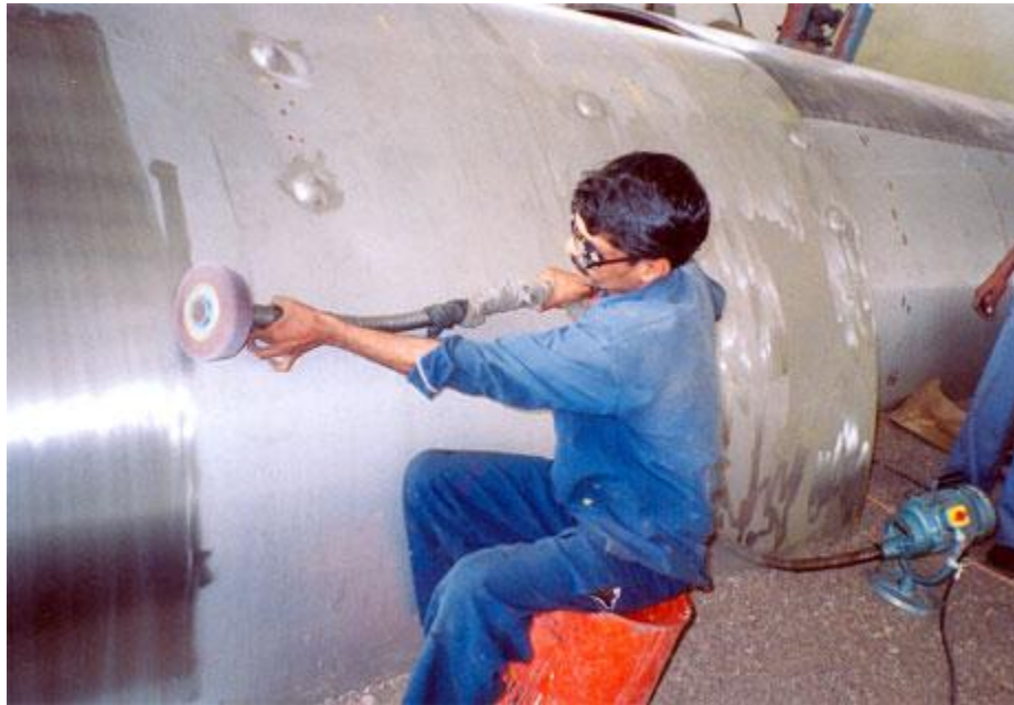
Figure 8.1 – A Buffing Operation In Action
