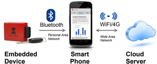
Figure 1. An example MGC application distributes logic and user interaction across embedded device, mobile phone and a cloud server.
