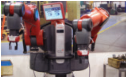
Fig. 15 — Rethink Robotics designed its robot so anyone could program it and so people could work near it without the need for a safety cage.
