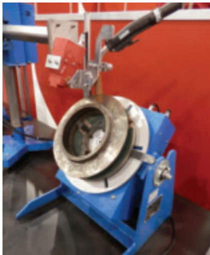
Fig. 17 — A new design in LD-600R, a portable multipurpose positioner, reduces the impact of noise generated during GTAW ensures stable rotation.
