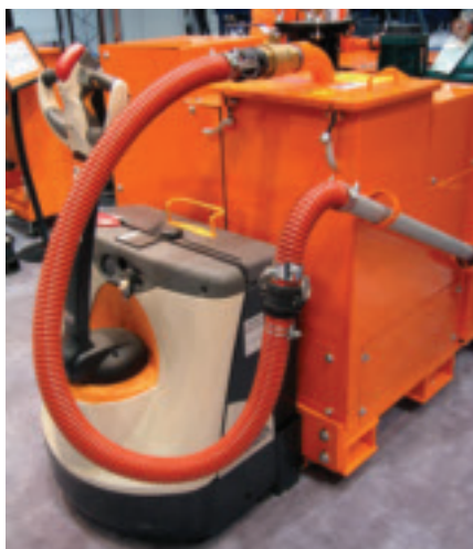
Fig. 8 — An attached motorized pallet facilitates moving the Eriez® SumpDoc to different locations.
