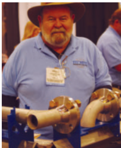
Fig. 13 — The FIT RITE pipe fitting system, shown here with its inventor Kayworth Mann, provides flange alignment and bolt hole orientation in seconds and can be used in the shop or field.
