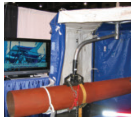
Fig. 10 — A lightweight support attaches directly to the pipe to hold the Hex-Hut shelter.
