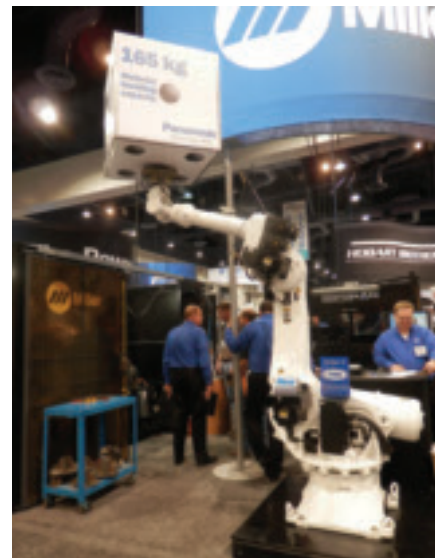
Fig. 19 — The G3 material handling robots, combined with Panasonic's G3 welding robot, position the material for optimum welding.
