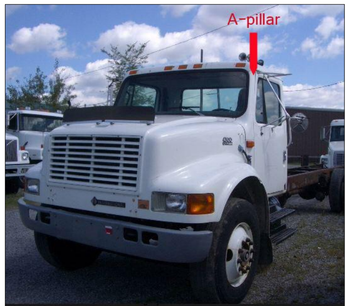
Exhibit 1. 1999 International 4700 truck cab, showing front "A" pillar
