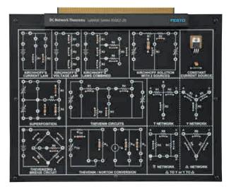
Consisting of nine training circuit blocks and a constant-source current block, the DC Network Theorems Circuit Board enables students to perform practical exercises that demonstrate theoretical DC principles. When a circuit has two voltage sources in different branches, theorems are used to solve for voltage and/or current in these circuits where Ohm's Law cannot be applied.
