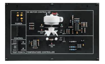
This Circuit Board is an add-on to the 32-Bit Microprocessor (Model 91017). It allows students to study how microprocessors can control and communicate with external devices. The Application Board has two application circuits: a DC Motor Controller, and a Temperature Controller.
