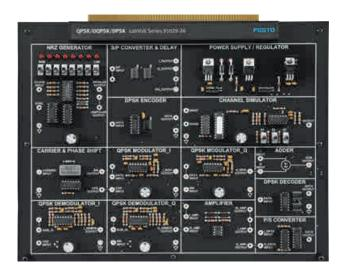
Phase-shift keying (PSK) is a method of digital communication in which the phase of a transmitted signal is varied to convey information. The QPSK/ OQPSK/DPSK board provides students with the theory and measurement skills required to implement and test different types of PSK modulation and demodulation techniques used in pulse-coded modulation (PCM) schemes.
