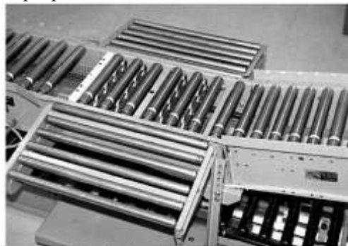
Figure 5.34 Pop-up belt. (Courtesy of Ermano, Inc.)
