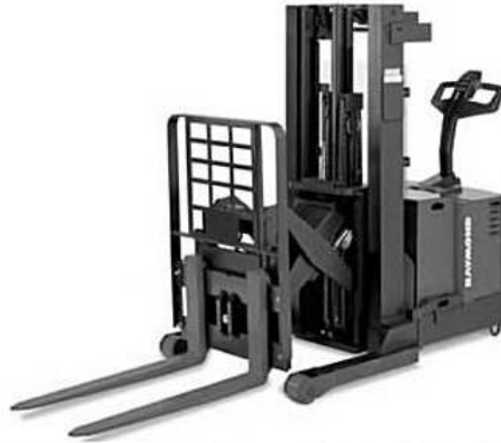
Figure 5.43 Walkie reach straddle truck. (Courtesy of Raymond Corp.)
