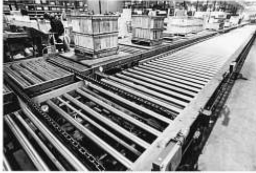
Figure 5.35 - Pop-up chain. (Courtesy of Eaton DHS.)
