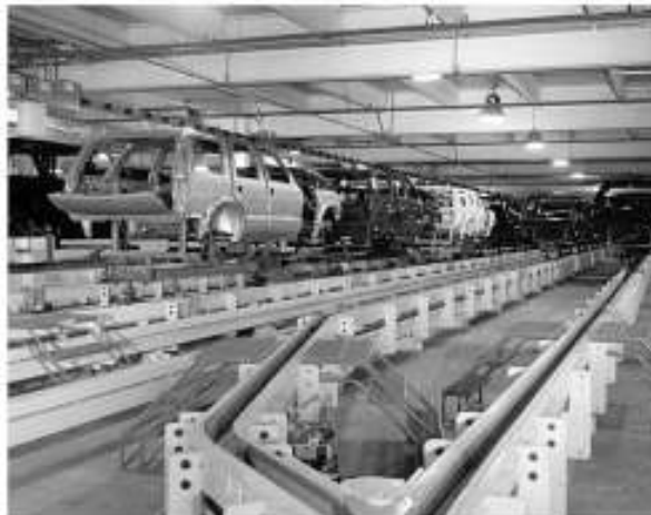
Figure 5.28. Powered push and free conveyor. (Courtesy of Jervis H. Webb Co.)
