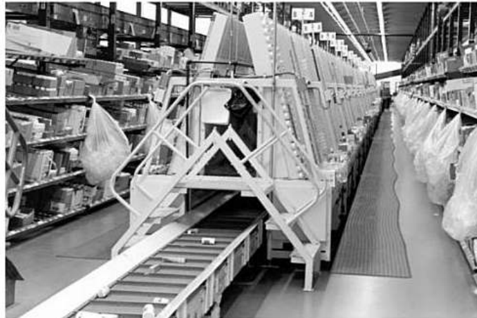
Figure 5.92 Automatic dispenser. (Courtesy of SI Systems, Inc.)
