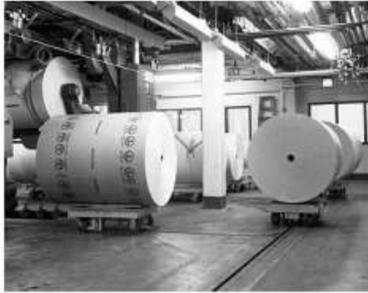
Figure 5.26. Tow line conveyor. (Courtesy of Jervis H. Webb Co.)
