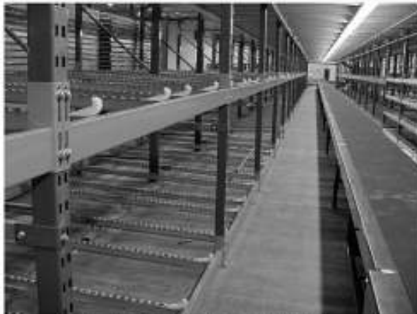
Figure 5.69 Pallet flow rack. (Courtesy of UNARCO, Inc.)
