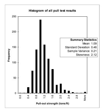
Figure 2-2. Histogram showing the distribution of pull-out strengths for all data collected in study.
