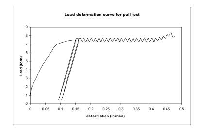
Figure 2-10. Load-deformation curve for a pull test carried out on a 5 ft. SS39 immediately after installation. The bolt was loaded until initial slippage, unloaded and reloaded twice and then pulled out of the hole for a a full 0.5 inches. Note that an approximately constant load of 7.5 tons was reached. From Scott, 1977.
