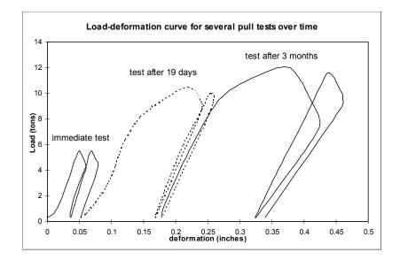
Figure 2-17. Load-deformation curves for three pull test carried out on the same 5 ft. SS39 bolt in hard shale: at the time of installation, at 19 days and at 3 months. From Scott, 1977.
