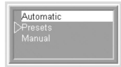
The hollow cursor means the operator cannot select this state.
