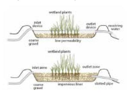
Fig. 4: CWs types: (a) FWS, (b) VF (Vymazal and Kröpfelová, 2009).
