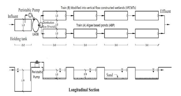
Fig (5) Vertical flow constructed wetlands (Train B).
