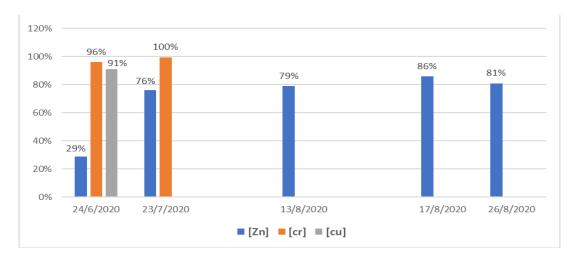
Fig (18): Zinc, chromium and cupper removal efficiency in CW1 with time
