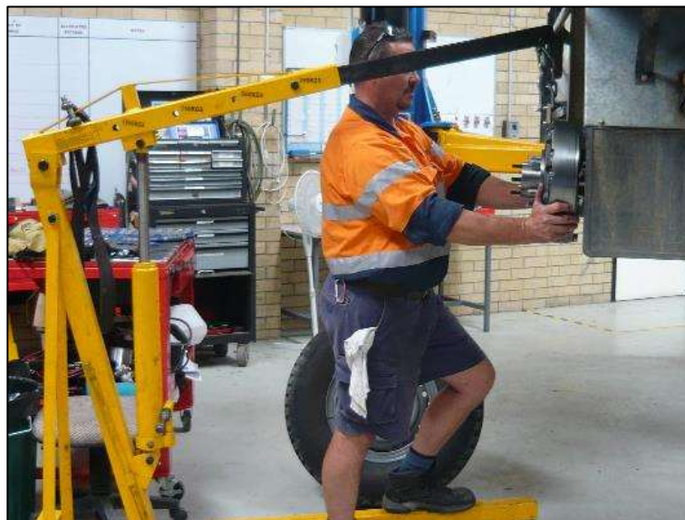
Figure 18: Carefully fit brake assembly over stub axle.
