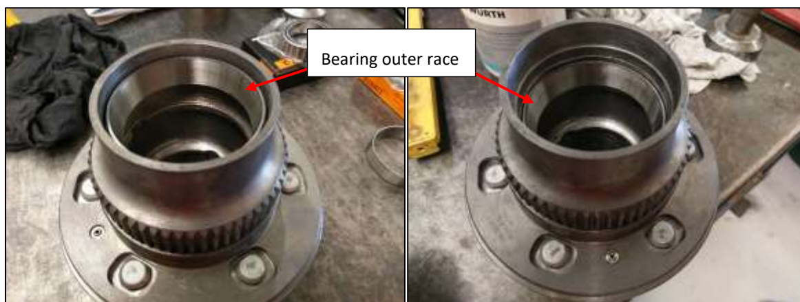
Figure 59: Bearing outer race in loose (left) and seated (right)
