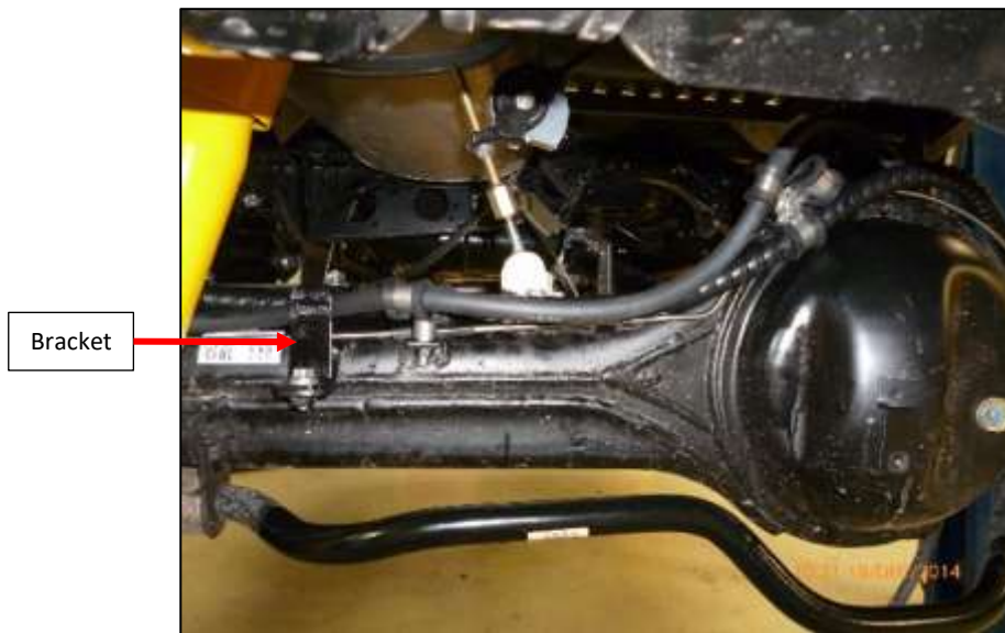
Figure 47: Brake lines routed on to LH brake unit (facing front of vehicle).
