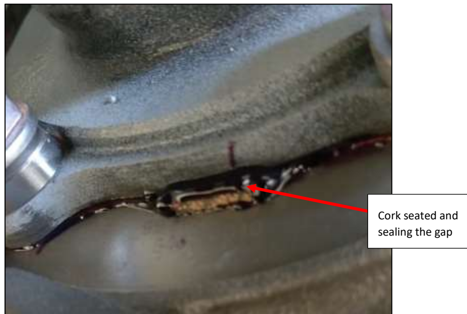
Figure 17: Cork part of the gasket in the slot.
