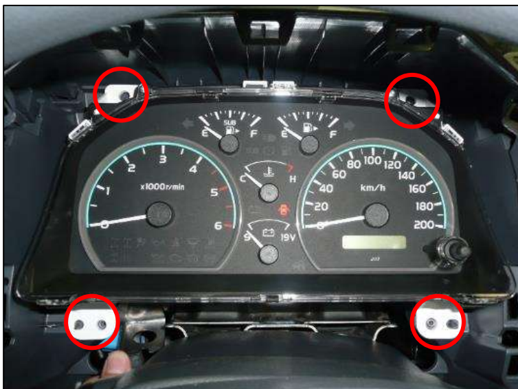
Figure 1: Instrument cluster retaining screws.
