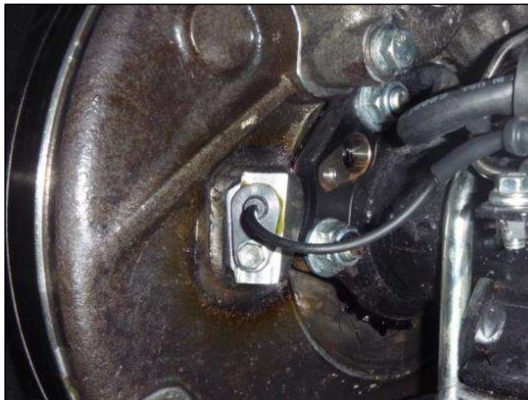
Figure 28: ABS harness installed in LH ABT™ Failsafe brake.
