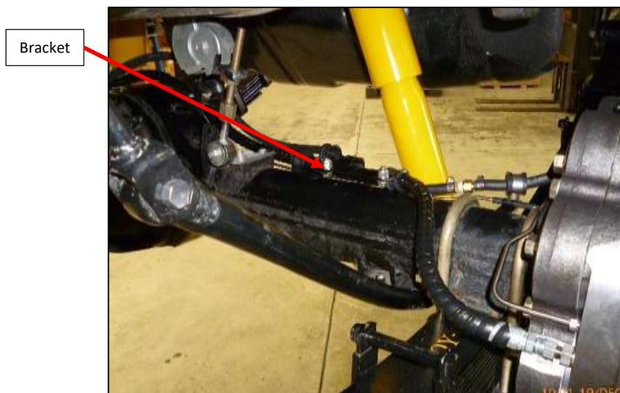
Figure 46: Brake lines routed on to LH brake unit (facing rear of vehicle).
