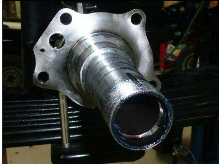
Figure 13: Clean axle flange and prepare gasket face.
