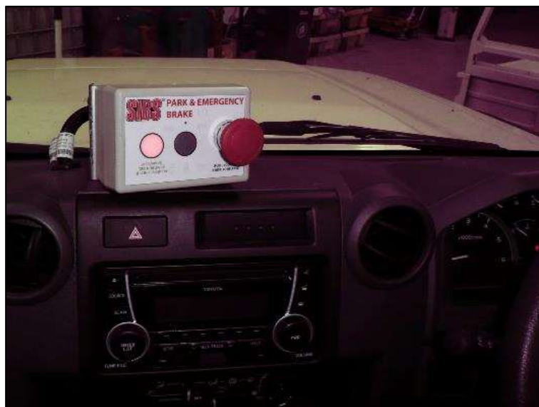
Figure 4: ABT™ Failsafe control unit mounted on dash.
