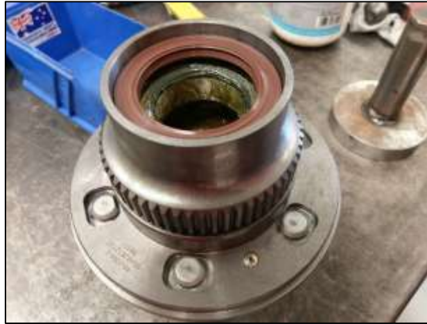
Figure 60: Shaft seal installed
