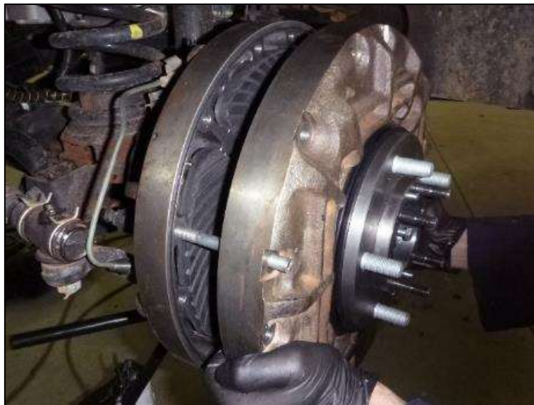
Figure 33: mounting the outer housing
