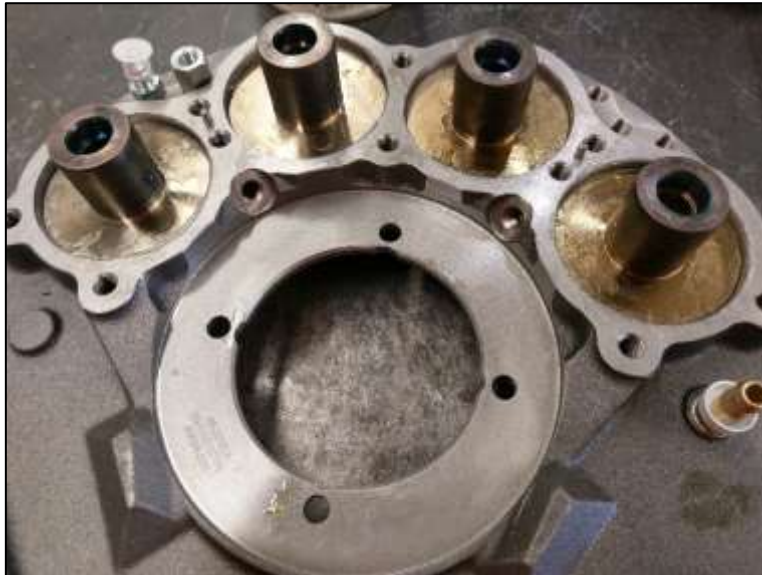
Figure 69 – Pistons installed in position
