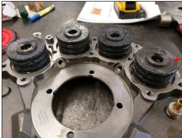
Figure 65: Lubricated springs on the pistons
