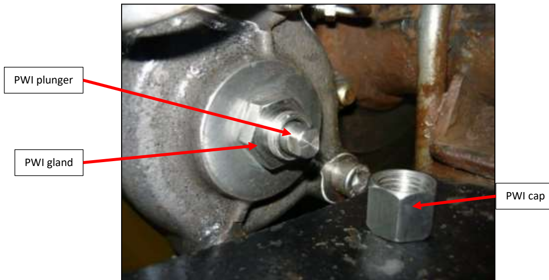
Figure 21: Pad wear indicator install in spring cover.
