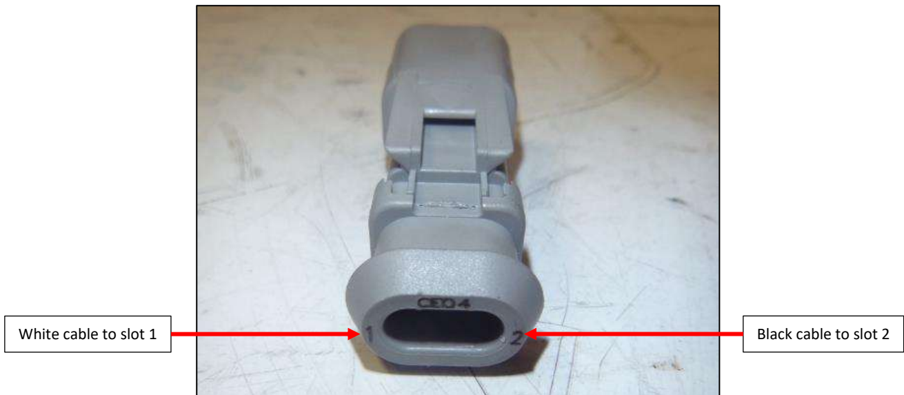
Figure 27: ABS harness connector.
