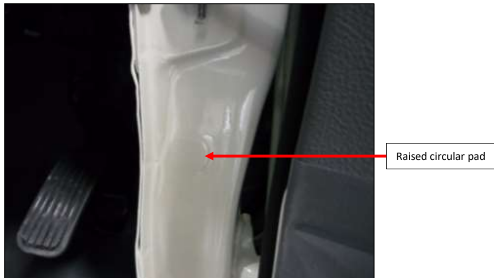
Figure 5: Proximity switch mounting location on A-pillar.
