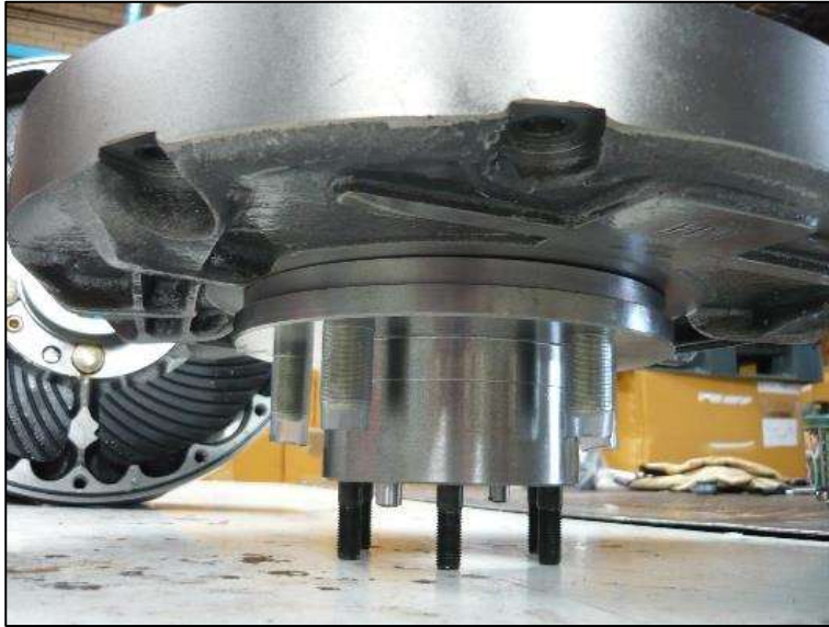
Figure 56: Outer housing, rotor and hub assembly.
