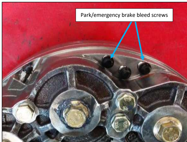
Figure 50: Park/emergency brake bleed screws.
