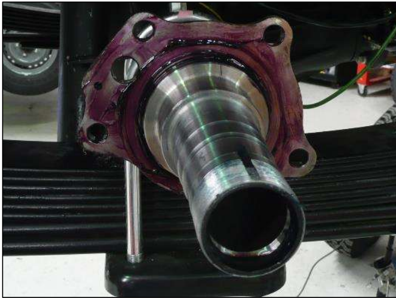
Figure 15: Apply Loctite® 515™ to axle flange.
