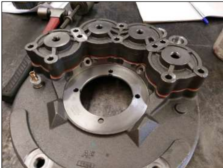
Figure 66: Spring cover in place with gasket
