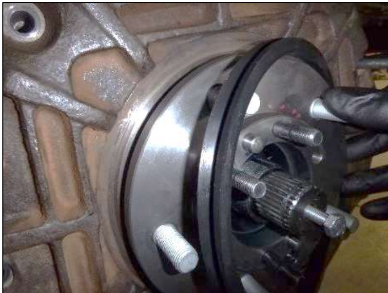
Figure 20: Fit V-lip seal over hub.
