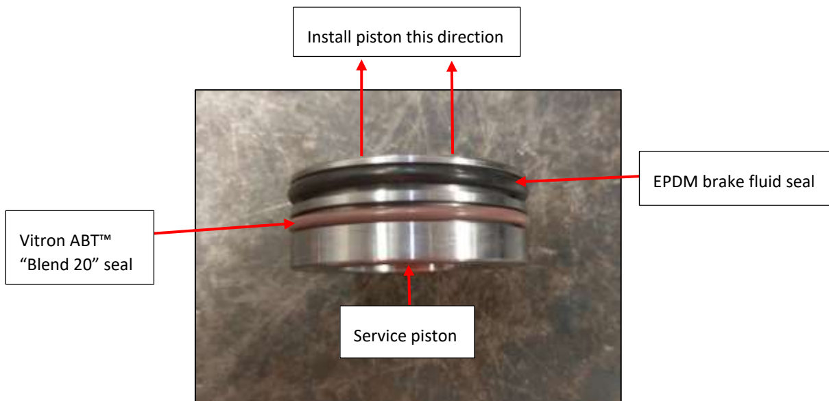
Figure 70: Piston O-ring positions
