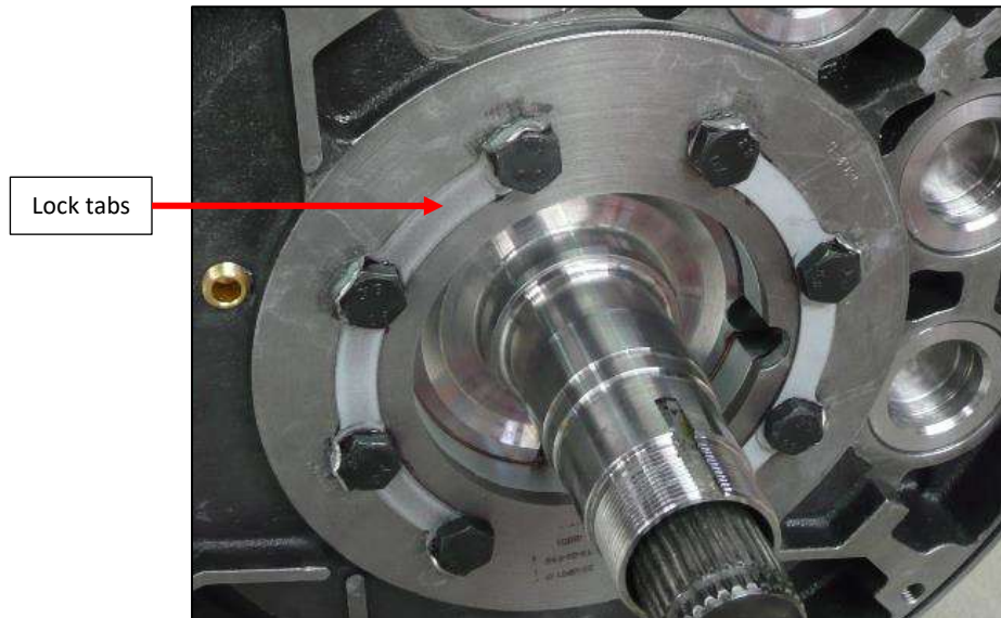
Figure 31: Install mounting bolts
