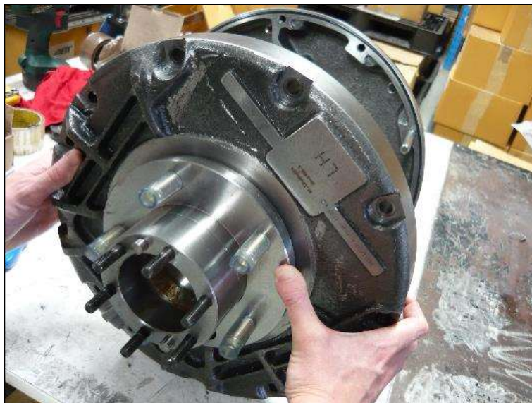
Figure 55: Separate inner and outer housings.
