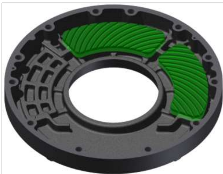
Figure 62: Brake pad position
