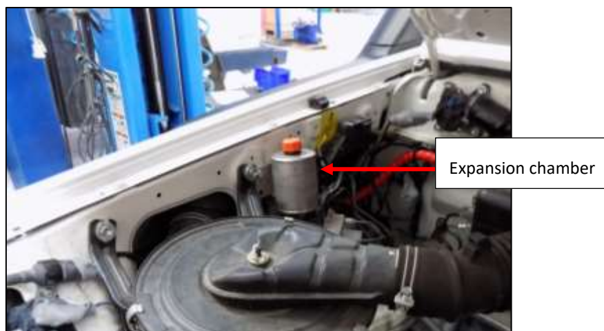
Figure 38: expansion chamber in the engine bay
