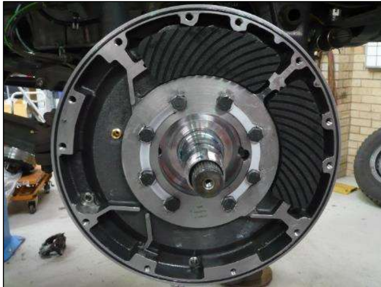
Figure 32: brake pads installed
