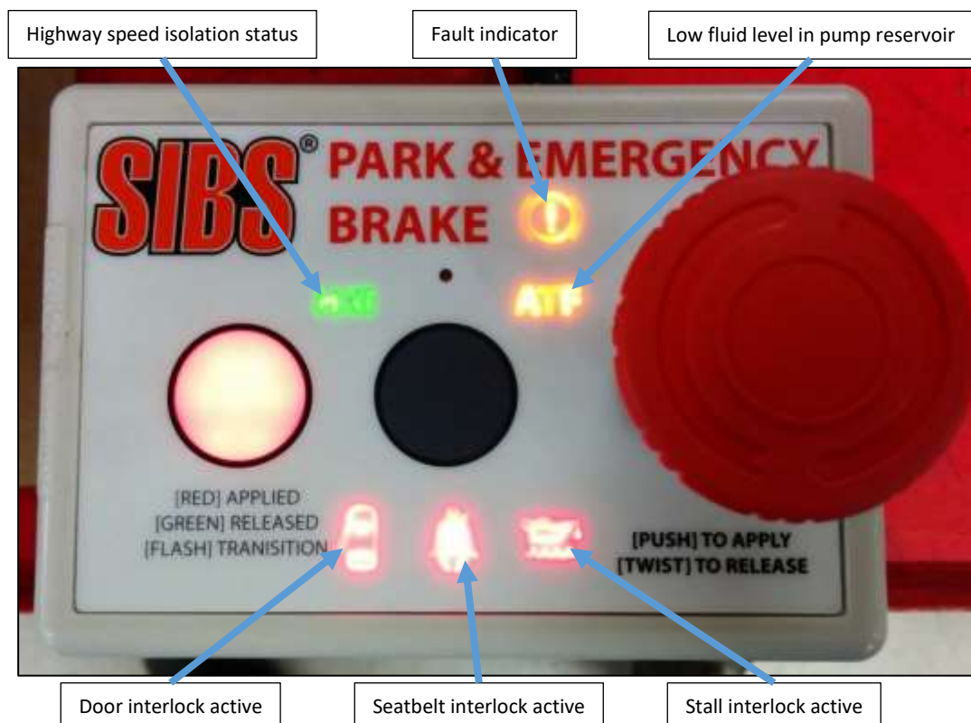
Figure 52: ABT™ Failsafe control unit warning lights
