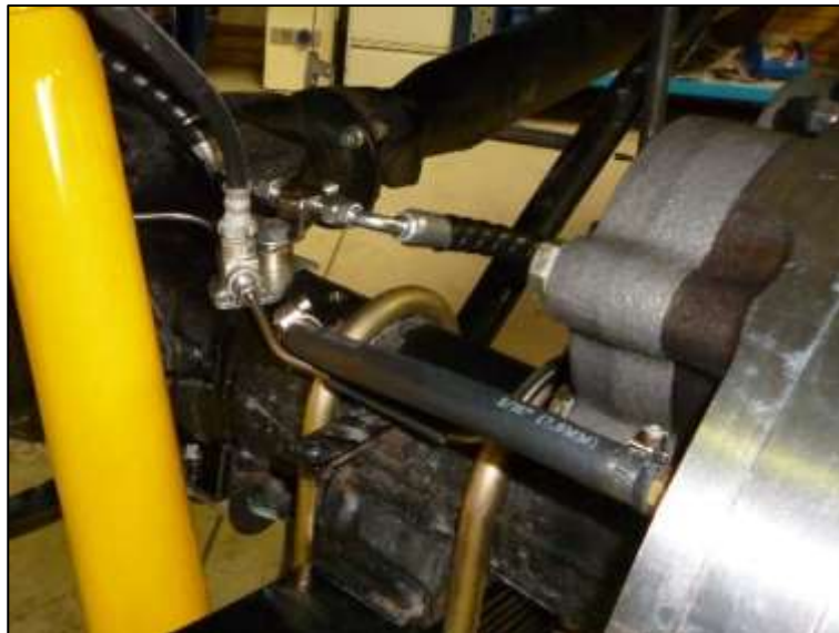
Figure 44: Brake lines routed on to RH brake unit (facing front of vehicle).
