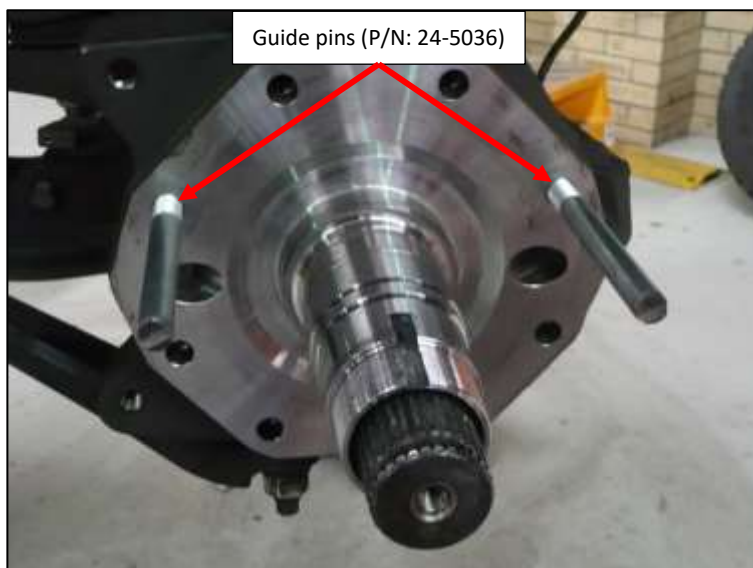
Figure 29: cleaned axle flange.
