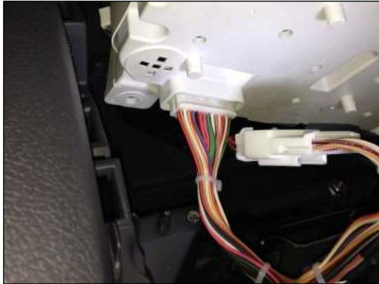
Figure 8: Connect the vehicle interface harness between the instrument cluster and 28-pin white OEM plug.
