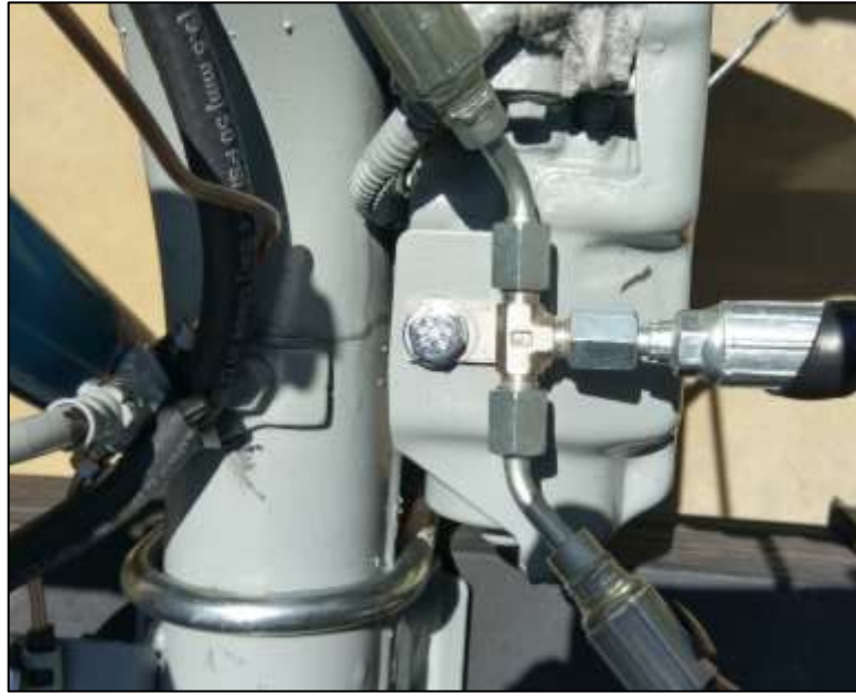
Figure 41: Differential lock tee-union location
