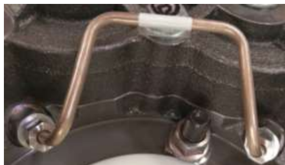
Figure 14 - Brake link pipe.
