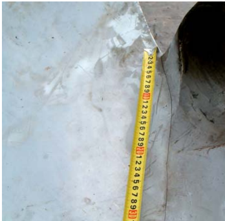
Fig.2 The crack on the pressure side
