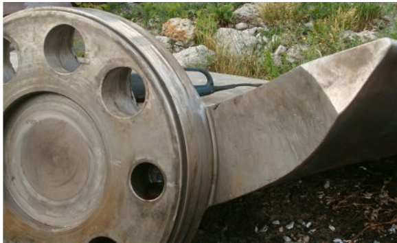
Fig.1 The cracked runner blade
