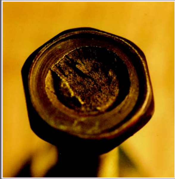
Fig. 3 As-received fractured bolt (M-1; M, mausoleum located in Michigan)
