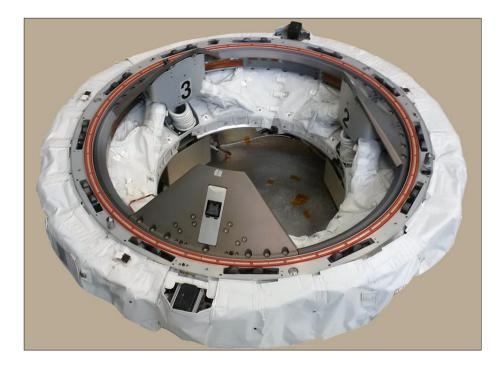
The program known as the International Low Impact Docking System (iLIDS) required several quad-bridge tension and compression miniature load cells to detect, guide, and dock incoming space vehicles. These load cells were to follow specific space and flight standards, ensuring their conformity with various forms of spacecraft.
