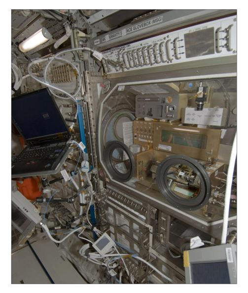
FUTEK participated alongside NASA and MIT in a joint venture to create the Shere History Extensional Rheology Experiment (SHERE). This program was designed to examine the stress and strain of polymer fluid in microgravity. The purpose of the study was to provide data that would help the development of in-situ fabrication and repair technology, a critical element in the evolution of autonomous exploration capability.
