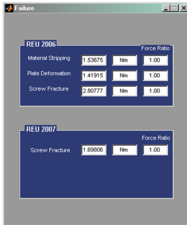
Figure 2.6: Failure GUI programmed with the failure model from CIMS REU 2006 and REU 2007
