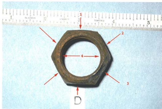
Photograph 1 Measurements 1 -3, across wrench flats, and measurement 4, minor internal diameter, performed on the lug nut specimens
