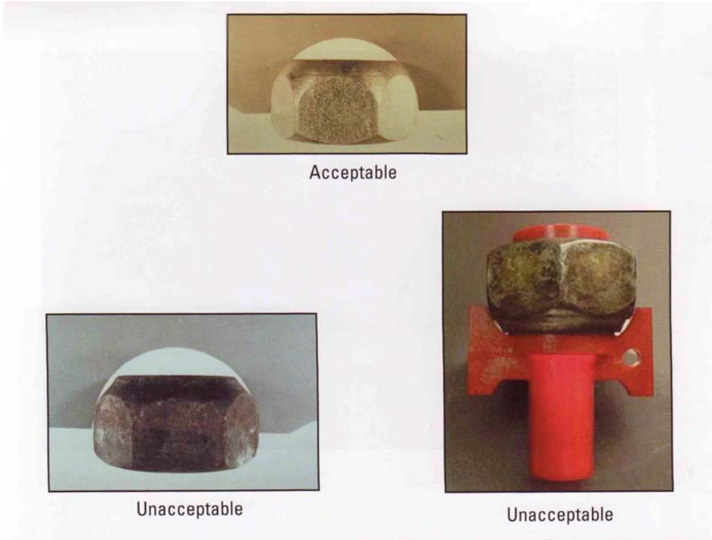
Figure 7-14. Users Guide p98 - Ball Seat Radius LowRes.jpg
