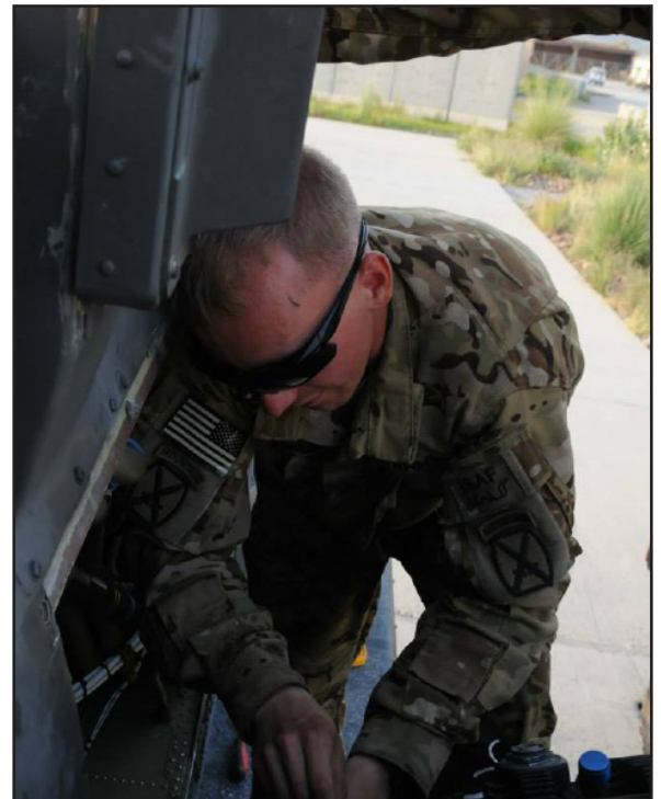
Pfc. Jess VanBuren, an AH-64 Apache helicopter repairer assigned to B Company, 1st Attack/Reconnaissance Battalion, Task Force Tigershark, 10th Combat Aviation Brigade, loosens a bolt in preparation to remove the number 2 engine gear box Sept. 6, at Forward Operating Base Salerno in Khowst Province, Afghanistan. (Photo by Staff Sgt. Todd Pouliot, 10th CAB)
