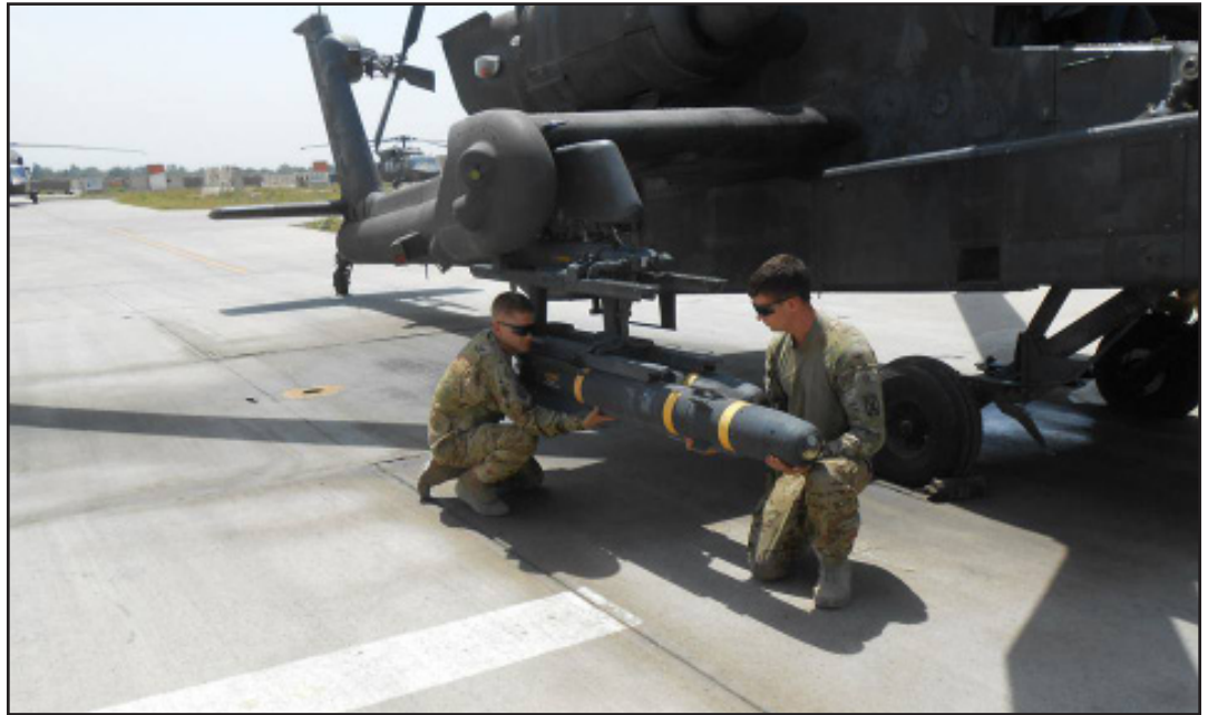
Spc. Shane Montgomery and Spc. Ethan Burke, AH-64 Apache helicopter armament, electrical, avionic, systems repairers assigned to Task Force Tigershark, load an AGM-114 Hellfire missile after completing maintenance on the Apache. (Courtesy photo)
