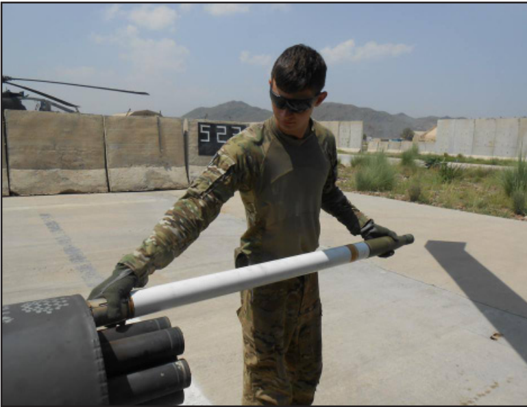
Spc. Ethan Burke, an AH-64 Apache helicopter armament, electrical, avionic systems repairer assigned to Task Force Tigershark, loads 2.75-inch Folding Fin Aerial Rockets onto an Apache after maintenance. (Courtesy photo)
