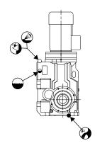
position for which it was ordered. See below for the placement of the vent, drain and oil level plugs based on drive size and mounting position. If it is necessary to mount the drive in a special orientation not shown below, including rotated and tilted drives, consult the Falk Corporation for changes necessary to provide proper lubrication. Refer to Table 9 for approximate quantities of oil by the drive mounting position.
