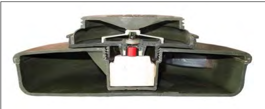
Figure 4 One of the C3B mines was sectioned to produce this training aid
