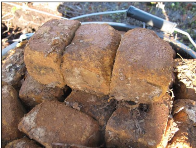
Figure C4 TNT charges from a booby trap in SA064. These appear to have been 400 g blocks of pressed TNT, wrapped in waxed paper. Pressed TNT is deemed 'cap sensitive', meaning that it can be initiated directly by a No 8 strength detonator. The edges of the blocks have been eroded but the bulk of the explosive remains intact. Historical data on TNT suggests that it can remain capable of detonation for several decades
