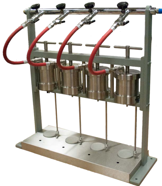
Figure 10-8 Four Unit Filter Press w/Manifold
