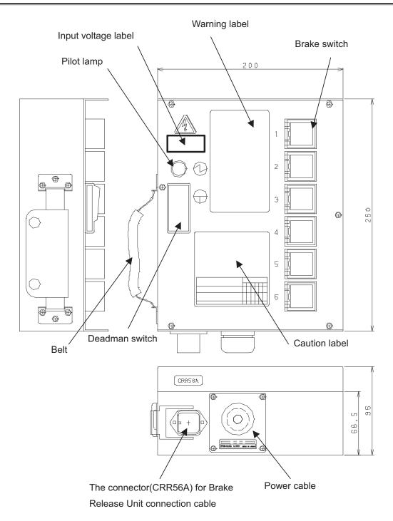
Fig.B.5 (a) Dimension of Brake Release Unit (Front view)
