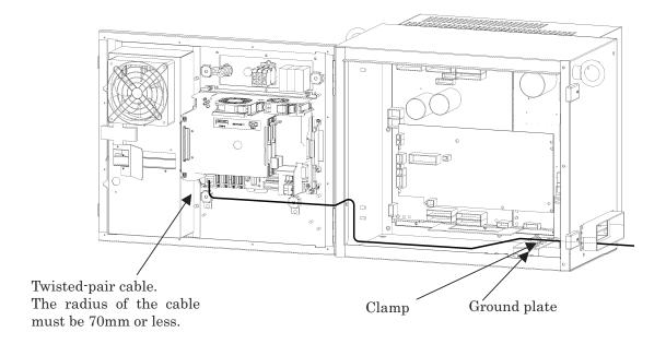
The Ethernet cable must be fastened by a cable clamp to prevent tension being applied to the modular connector (RJ-45) that connects the cable to the controller even if the Ethernet cable is pulled directly. This clamp is also used to ground the cable shield.
