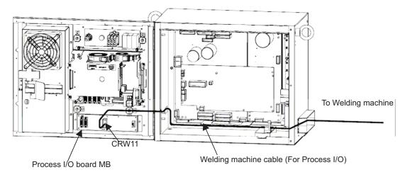
Fig. 4(c) Connecting the welding machine cable (Process I/O board MB)
