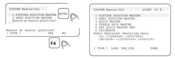
(7) Select "6 CALIBRATE" and press the F4 key (yes). Calibration is performed. Alternatively, to perform positioning, turn the power off, and then turn it on again. Calibration is performed whenever the power is turned on.
