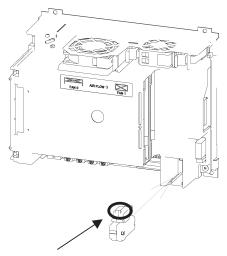
Insert the unit until the latch snaps into the case.
