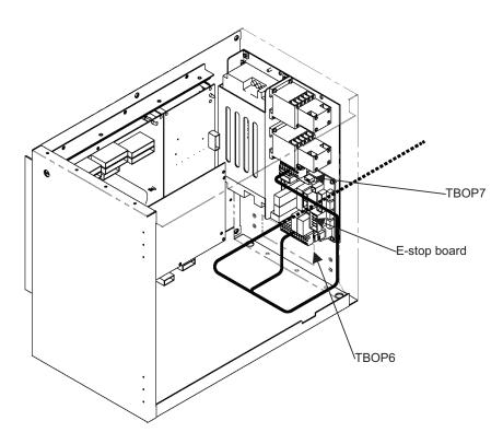
Fig.3.3.4 (a) Connection of the external emergency stop
