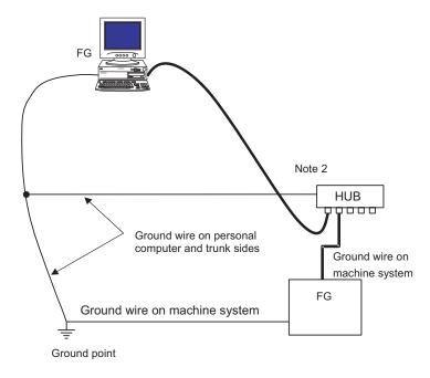
Fig. 4.8.2.5 (c) Wiring on a single ground point
