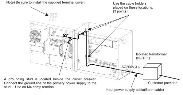
Fig.3.3.3 (b) Input power cable (ARC Mate 100iC, M-10iA, ARC Mate 120iC, M-20iA, ARC Mate 50iC)
