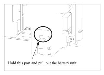
(5) Install a new battery unit. (Insert the battery unit until the latch of the unit snaps into the case.) Check that the battery unit is latched securely.
