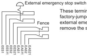
These terminals are factory-jumpered. When using external emergency stop inputs, remove the short-circuit plate.
