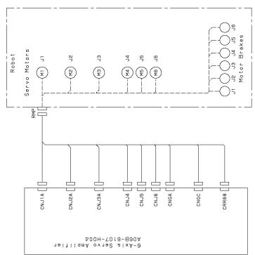
Fig. A (k) Motor power connection (ARC Mate 100iC, M-10iA)
