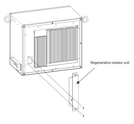
Fig. 7.3 (a) Regenerative resistor unit replacement (LR Mate 200iC, M-1iA)
