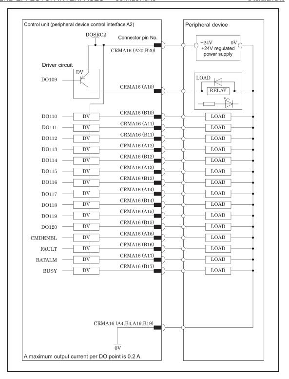
The following shows the connector interface of the optional peripheral device cables on the peripheral device side.
