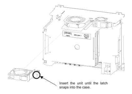
Fig.7.7 Replacing the control section fan motor
