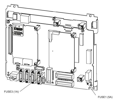
Fig.7.9.2 Replacing fuses in the main board
