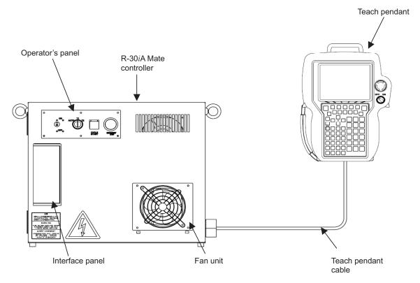
Fig.2.1 (a) External view of the R-30iA Mate controller
