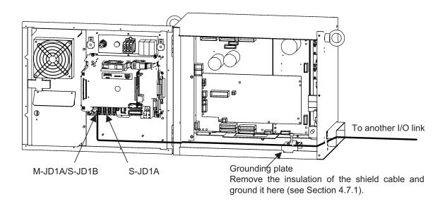
Fig. 3.2.2 (a) Path of the I/O link cable
