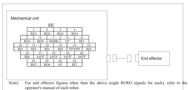
Fig. 4.4.2 Connection between the ARC Mate 100iC/M-10iA, ARC Mate 120iC/M-20iA and end effector
