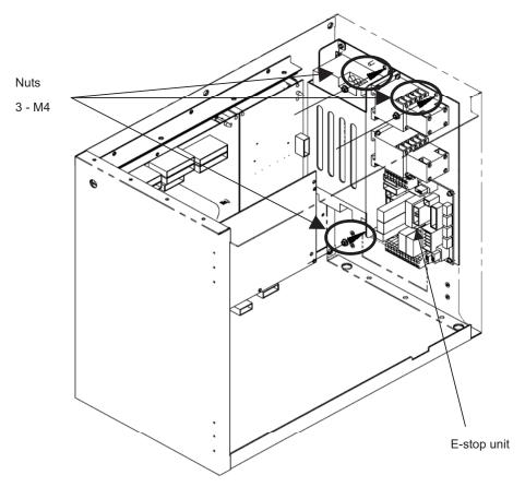
Fig.7.4 Replacing the emergency stop unit
