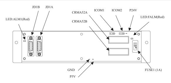
Fig.4.4 Process I/O board MA
