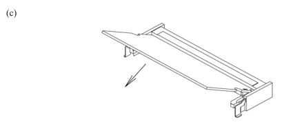
Fig.7.2 (c) Demounting/mounting a module
