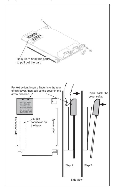
Fig. 7.2 (a) Demounting the card on the main board
