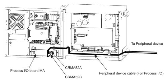
Fig. 4(b) Connecting the peripheral device cable (Process I/O board MA)
