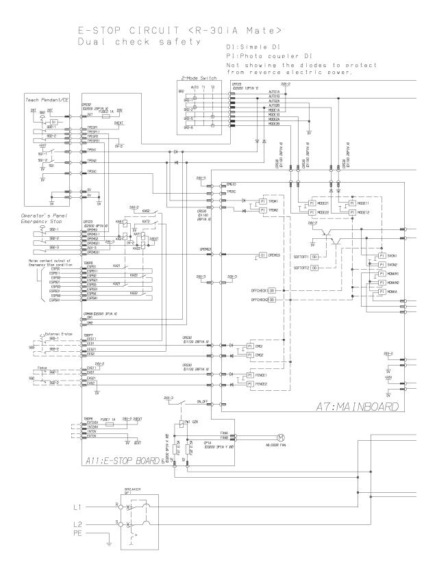
Fig. A (c) Emergency stop circuit diagram (M-1iA, LR Mate 200iC)
