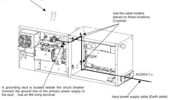
Fig.3.3.3 (a) Input power cable (LR Mate 200iC, M-1iA)
