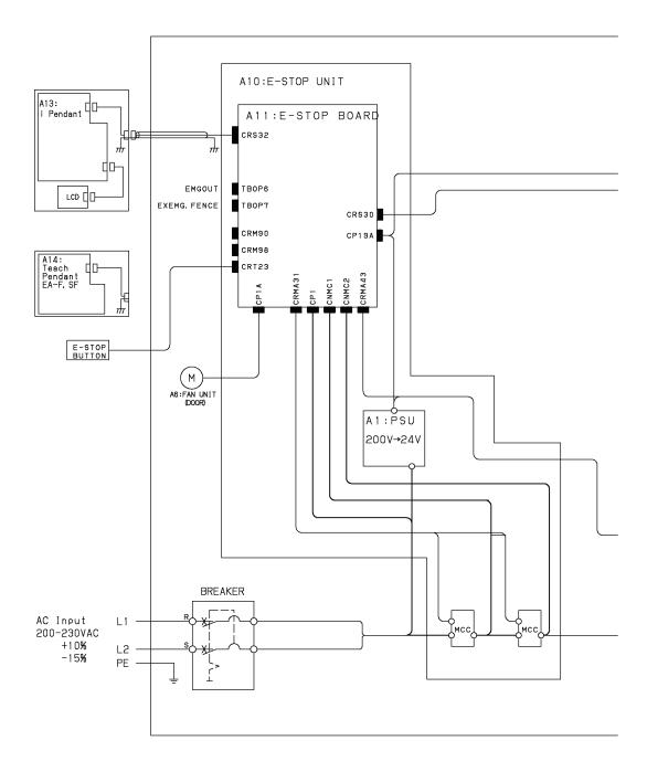
Fig. A (a) System block diagram (M-1iA, LR Mate 200iC)
