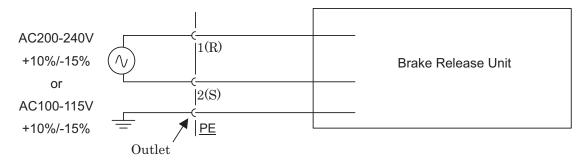
Fig.B.4 How to connect the plug to the power cable
