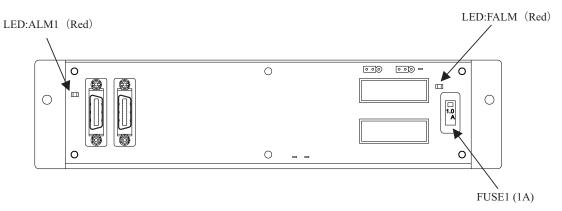
Fig.3.7 (d) LED status on the process I/O board MA
