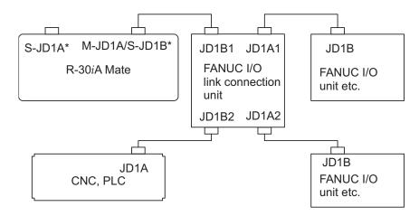
3. When the R-30*i*A Mate controller is used as an I/O link slave (When a CNC or PLC is the I/O link master)
