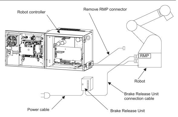
Fig.B.3 (b) How to connect Brake Release Unit (In case of operating the Robot)
