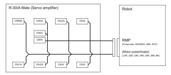
Fig. 3.3.1 Robot connection cable
