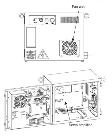
Fig.3.5 (ah) SRVO-291 IPM over heat
