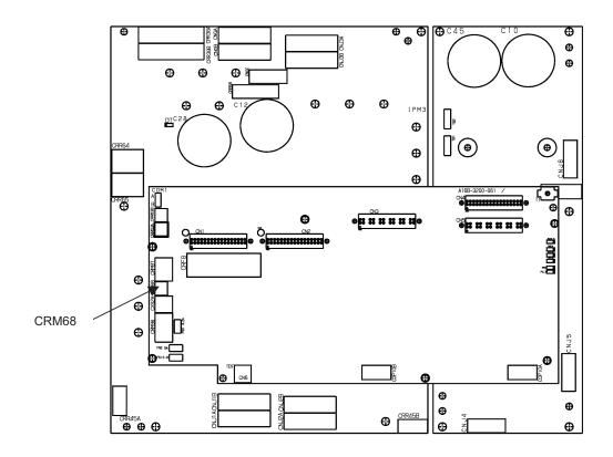
Fig.3.3.6 6-axis servo amplifier
