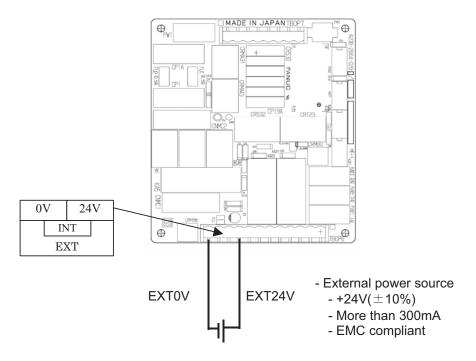
The relays for emergency stop input and output can be separated from controller's power. Please connect external +24V instead of internal +24V,if emergency stop output must not be effected controller's power.
