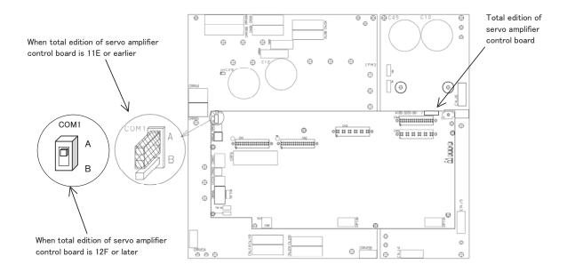
Fig.5.2 (a) Setting of servo amplifier
