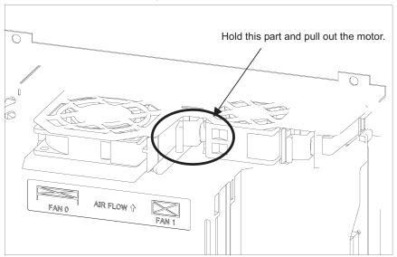
(3) Install a new fan unit. (Insert the unit until the latch of the unit snaps into the case.)
