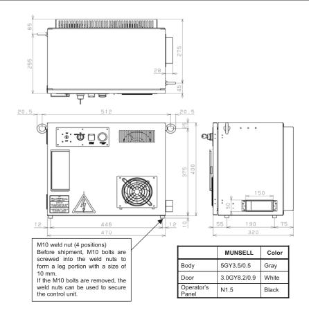
Fig. 5.2.1(c) External dimension (LR Mate 200iC, M-1iA)
