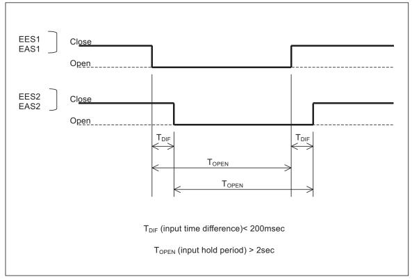
Fig. 3.3.4(c) Input timing of duplicate safety signals
