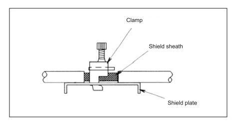
For noise protection, cut part of the jacket of the peripheral device cable to expose the shield sheath, and fasten this part to the shield plate with the clamp.
