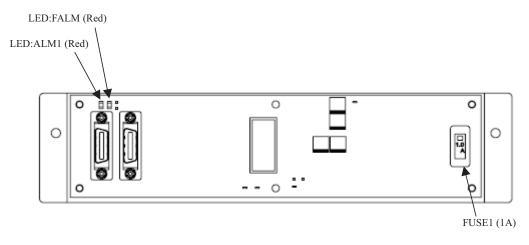
Fig.3.6 (e) Fuse on the process I/O board MB
