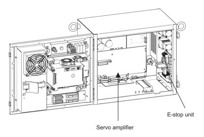
Fig.3.5 (t) SRVO-105 Door open or E-stop
