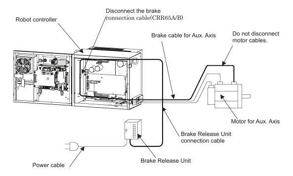
Fig.B.3 (c) How to connect Brake Release Unit (In case of operating the Aux. Axis)
