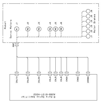
Fig. A (I) Motor power connection (ARC Mate 120iC, M-20iA)
