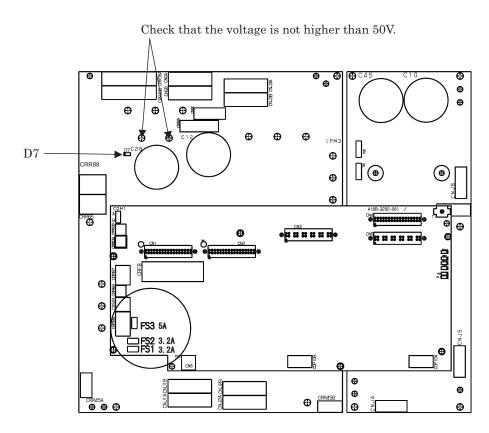
Fig.3.6 (b) Fuses on the servo amplifier
