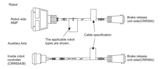
Fig.B.2 Brake release unit connection cable
