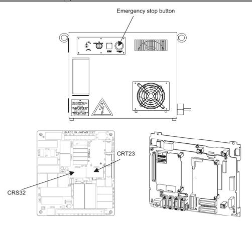
(E-stop board) (Main board) Fig.3.5 (a) SRVO-001 Operator panel E-stop
