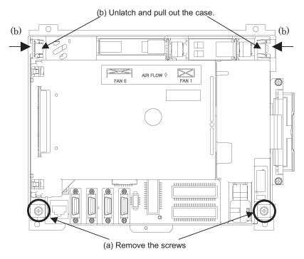
Fig.7.1.1 Replacing the backplane board
