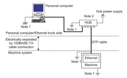
Fig. 4.8.2.5 (b) Small-Scale Network
