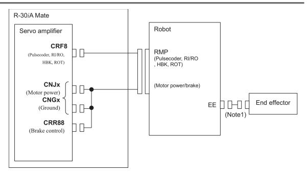
Fig.3.1 (a) Mechanical connection diagram
