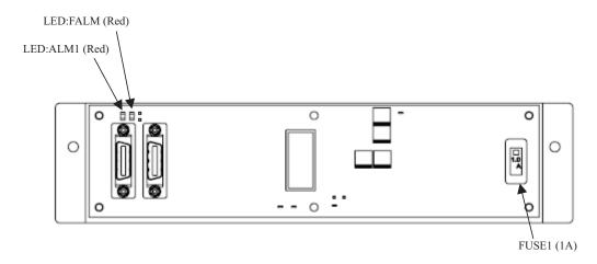
Fig.3.7 (e) Fuse on the process I/O board MB
