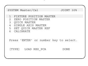
(5) Move the robot by jog feed to the mastering position. Release the brake on the manual brake control screen if necessary.
