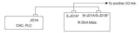
\* M-JD1A/S-JD1B: For main board general versions equal to or earlier than 04A, the connector name is JD1A.
