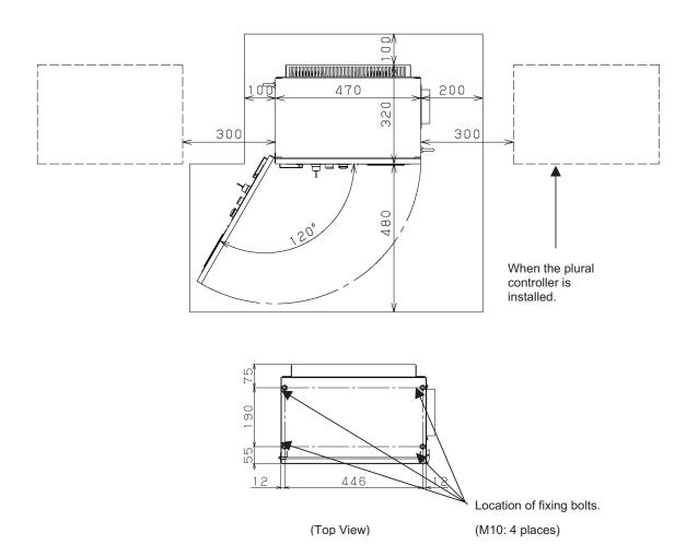
Fig. 5.2.1 (a) Installation dimension (LR Mate 200iC, M-1iA)
