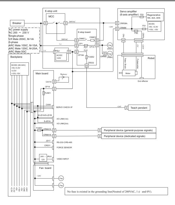
Fig. 6.1 Block diagram of the power supply
