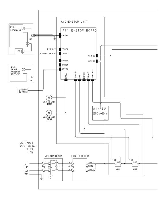
Fig. A (b) System block diagram (ARC Mate 120*i*C, M-20*i*A, ARC Mate 100*i*C, M-10*i*A, ARC Mate 50*i*C)
