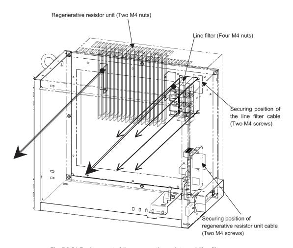
Fig. 7.3 (b) Replacement of the regenerative resistor unit/line filter (ARC Mate 100*i*C, M-10*i*A, ARC Mate 120*i*C, M-20*i*A ARC Mate 50*i*C)
