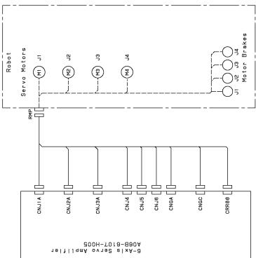
Fig. A (j) Motor power connection (M-1*i*A/0.5S(4-Axis))
