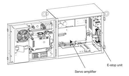
Fig.3.5 (m) SRVO-045 HCAL alarm SRVO-046 OVC alarm
