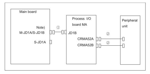
(Note) The connection depends on whether the R-30*i*A Mate is the I/O link master or an I/O link slave. For details, see Section 3.2.1.
