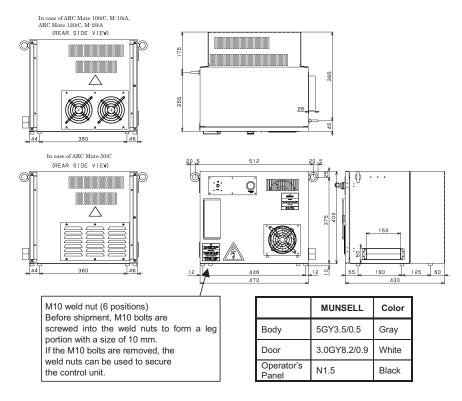
Fig. 5.2.1(d) External dimension (ARC Mate 100iC, M-10iA, ARC Mate 120iC, M-20iA, ARC Mate 50iC)
