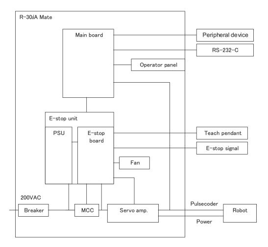
Fig.2 Block Diagram of Electrical Interface Connection
