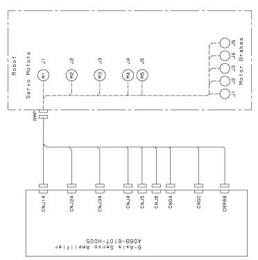
Fig. A (i) Motor power connection (LR Mate 200iC(5-Axis))
