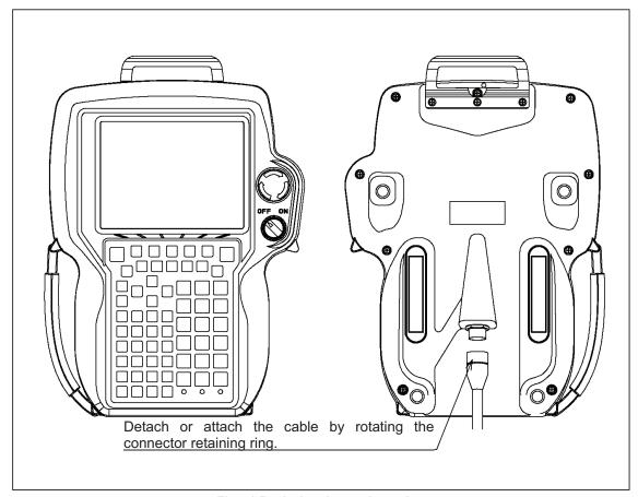
Fig.7.6 Replacing the teach pendant
