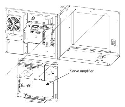
Fig.7.5 (b) Replacing the Servo amplifier
