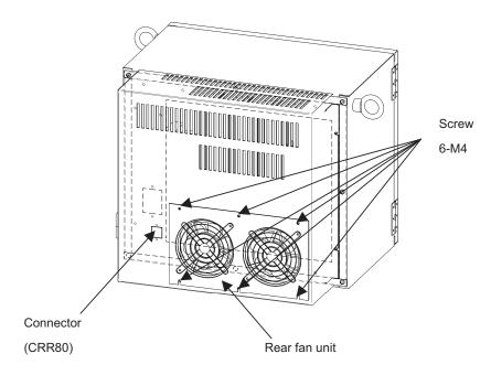
Fig.7.8.1 (c) Replacing the rear fan unit
