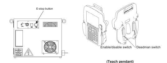
Fig.3.5 (ae) SRVO-233 TP disabled in T1, T2/Door open SRVO-235 Short term Chain abnormal
