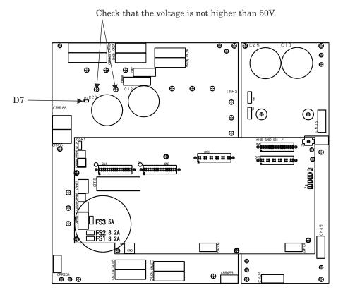
Fig.7.9.1 Replacing fuses in the servo amplifier
