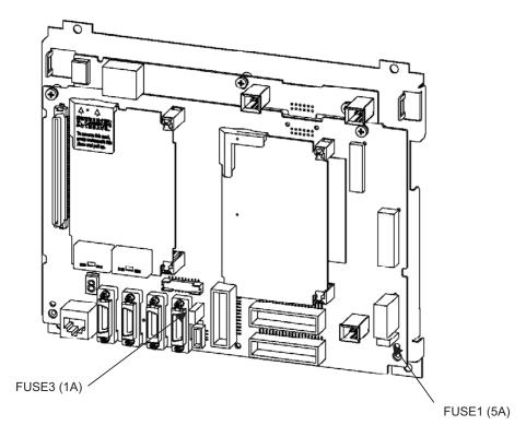
Fig.3.6 (a) Fuses on the main board
