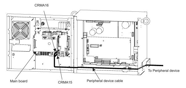
Fig. 4(a) Connecting the peripheral device cable (CRMA15, CRMA16)
