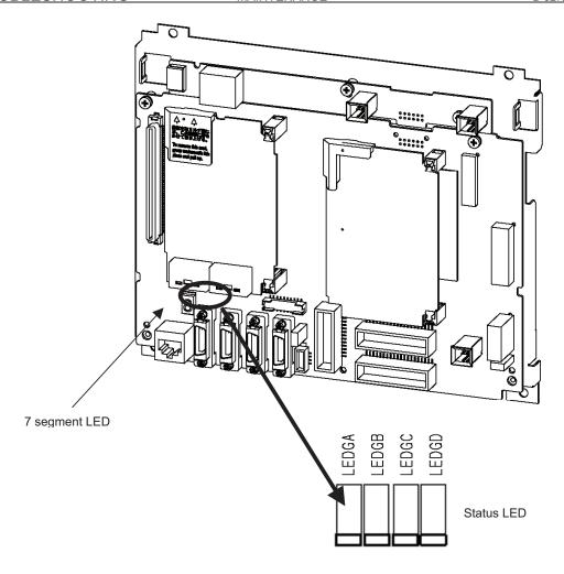
Fig.3.7 (b) LED status on the main board
