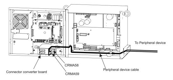
Fig. 4(d) Connecting the peripheral device cable (Connector converter board)
