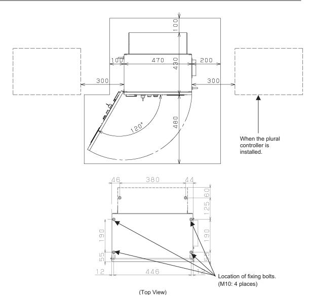
Fig. 5.2.1 (b) Installation dimension (ARC Mate 100iC, M-10iA, ARC Mate 120iC, M-20iA, ARC Mate 50iC)
