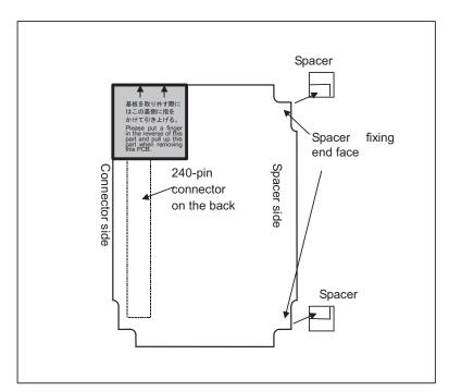
Fig. 7.2 (b) Mounting the card on the main board
