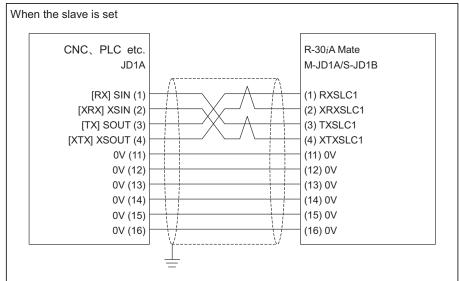
Fig. 3.2.2 (b) Connection diagram of I/O Link cable
