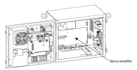
Fig.3.5 (r) SRVO-059 Servo amp init error SRVO-070 STBERR alarm
