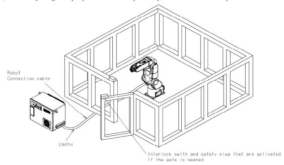
Fig.1.2 Safety fence and safety gate
