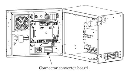
Fig.4.6 Location of the Connector converter board
