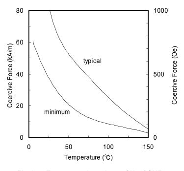
Fig. 6-7 Temperature dependence of Hc of GMF
