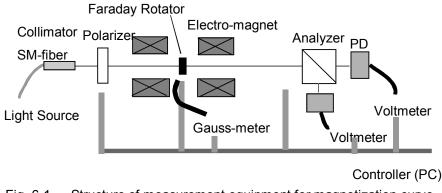
Fig. 6-1 Structure of measurement equipment for magnetization curve
