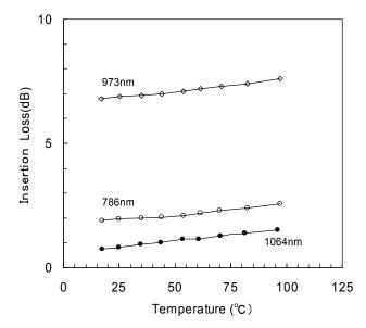
Fig. 5-16 Temperature dependence of insertion loss of GLB in short wavelength
