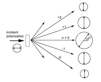
Fig. 5-19 Diffraction by multi-domain structure
