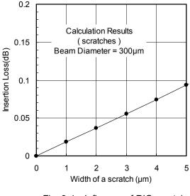
Fig. 9-4 Influence of RIG scratch on insertion loss
