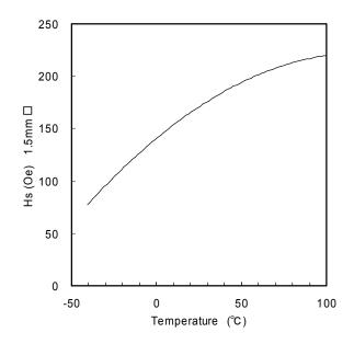
Fig. 6-4 Temperature dependence of saturation field of GSF
