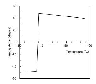
Fig. 6-9 Change in sign of Faraday rotation angle near compensation temperature with external magnetic field
