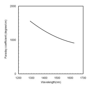
Fig.4-3 Wavelength dependence of Faraday coefficient
