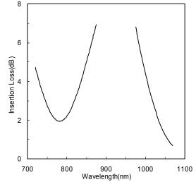
Fig.5-14 Insertion loss of GLB in short wavelength
