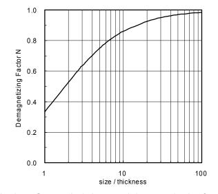
Fig. 6-5 Geometrical shape and demagnetization factor
