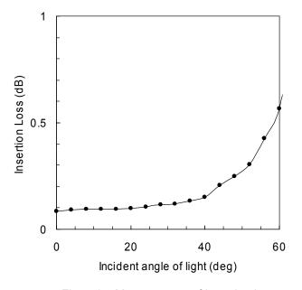
Fig. 5-9 Measurement of insertion loss
