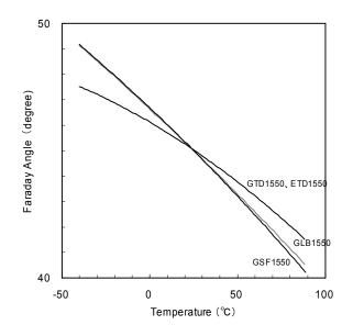
Fig.5-5 Temperature dependence of Faraday rotation angle
