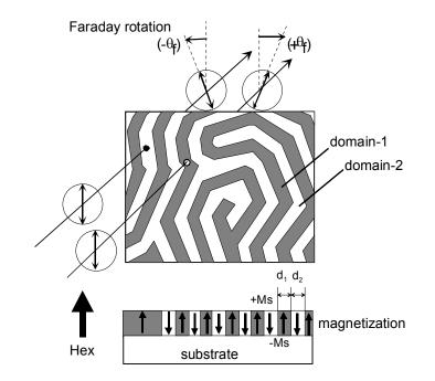
Fig. 5-17 Multi-domain structure and Faraday rotation of RIG
