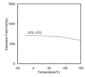
Fig. 6-3 Temperature dependence of saturation field of GTD and ETD
