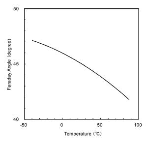
Fig.5-4 Temperature dependence of Faraday angle
