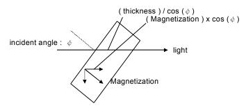
Fig. 5-7 Incident angle and magnetization
