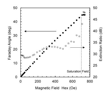
Fig. 5-18 Measurement of Faraday rotation angle and extinction ratio in multi-domain structure.
