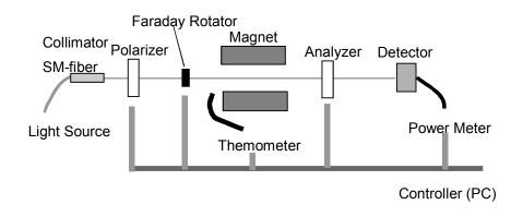
Fig.5-1 Measurement equipment for Faraday angle and extinction ratio
