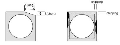
Fig. 9-5 Chipping and corner chip
