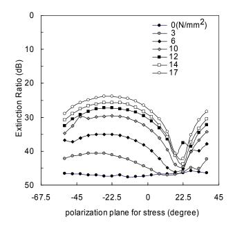
Fig. 5-11 Degradation in extinction ratio due to external stress
