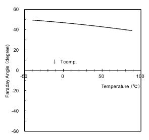
Fig. 6-10 Change in sign of Faraday rotation angle near compensation temperature without external magnetic field
