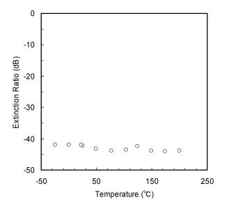
Fig.5-6 Temperature dependence of extinction ratio
