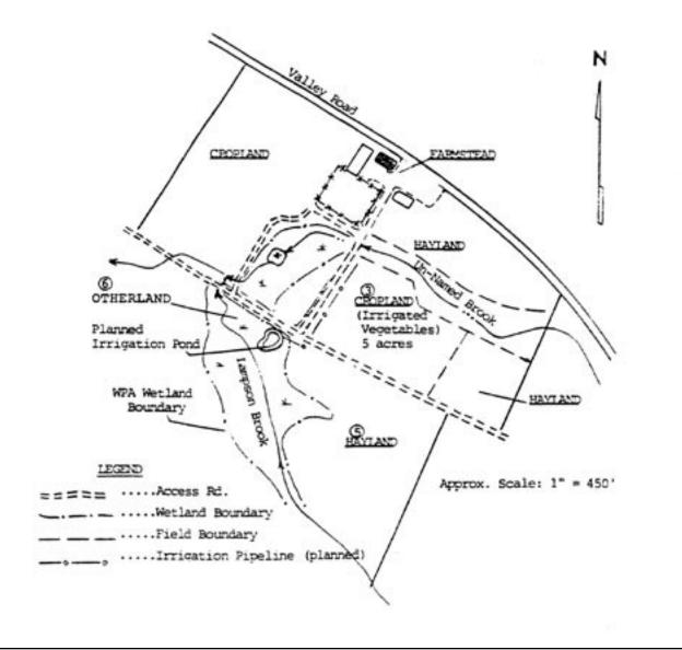
This plan was prepared to serve as a requirement under the "Conservation Plan Limited Project" permit category of the Massachusetts Wetlands Protection Act. The plan guides the establishment of a new Irrigation Pond within an area of Bordering Vegetated Wetland (BVW). The Pond will support Cropland Field No. 3 Irrigated Vegetables, 5 acres.
