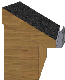
GUTTER LIP RUNNING INTO THE HOUSE
