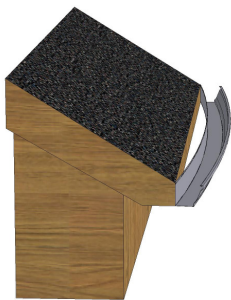
GUTTER RUNNING INTO THE HOUSE
