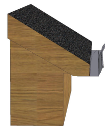
GUTTER LIP RUNNING AWAY FROM THE HOUSE
