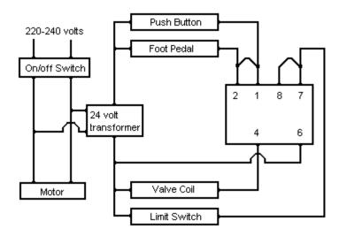
The on/off switch turns on power to both the electric motor and the valve coil control circuit. It must be 1 HP rated.
