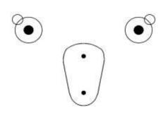
NOTE: The bending die must be fastened using the 2 securing hex bolts and must be kept tight at all times or injury to operator and/or damage to machine could result.
