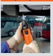
Even very large windows can be cut out from the interior using a type 081 cutter blade. Recommended speed: setting 3–5.
