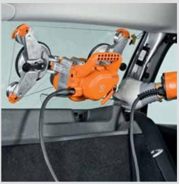
By removing the telescoping unit and installing the guide rollers directly on the drive unit, small side windows can also be removed without repositioning.
