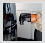
Type 207 and 209 L-shaped blades come into use on truck and bus windows with limited space between glass and frame. They will also cut through fixed strips easily and quickly. Recommended speed: setting 4–5.
