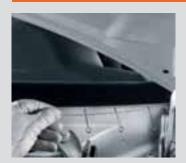
If the window extends over the body flange, use of metal pins is recommended so the wire is against the glass when cutting.
