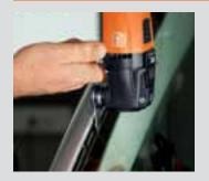
With the L-shaped blade, you get approximately 40% better cutting performance than with a comparable U-shaped blade operating at the same speed. Damage to the auto body is practically excluded. Recommended speed: setting 3–4.
