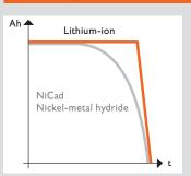
Powerful from first cut to last: the new FEIN lithium-ion technology provides constant power until the battery is completely drained.
