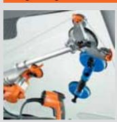
In rare cases the telescoping arm can slip on the window. This can be avoided with a normal suction lifting handle.
