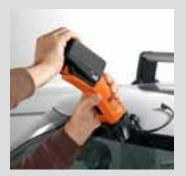
Encapsulated windshields and molded frames, including those with aluminum reinforcement, can be removed in one step using the L-shaped blade.
