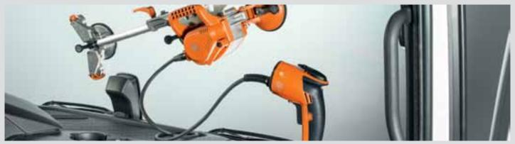
Truck windows can be safely removed with a single repositioning of the SUPERWIRE. The removal starts on the right side of the vehicle. This allows the window to be cut out to approximately the middle of the headliner. Then the SUPERWIRE must be moved to the left side.
