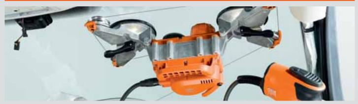
If the SuperWire cannot be mounted with the telescoping arms, it must be repositioned once. After insertion of the wire, the SuperWire is attached at the top right. The window is cut out as far as the upper edge and the SuperWire is then moved to the left in order to cut out the remainder of the window.
