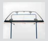
For the wire length, 5–6 times the overall width of the lower window edge is sufficient.
