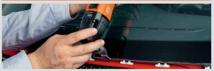
The U-shaped blades are used for glass removal below hood level. Recommended speed: setting 3-5.
