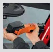
If the gap between glass and auto body is less than  $\frac{1}{2}$ " (3 mm), the windshield must be cut out from the interior using a straight blade. Recommended speed: max. setting 3.
