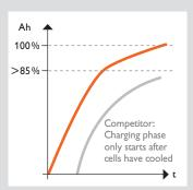
Short charging time: high quality cells with low internal resistance reduce warming and the battery does not need to be cooled down at exterior temperatures below 113°F.
