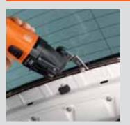
Side and rear windows are easily and quickly removed from the interior using the type 143 cutter blade and the adjustable depth stop. Recommended speed: max. setting 3.
