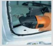
On some VW models the side and rear windows are equipped with glued-in frames. FEIN provides the answer to damagefree window removal on VW Passat wagons up to 2004, VW Polos up to 2001, Lupo, Seat and VW Golf III models.
