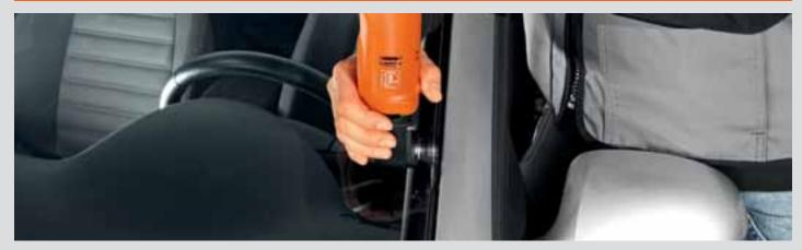
Extremely fast cutting: the type 207 L-shaped blade has an approximately 40% better cutting performance than a comparable U-shaped blade at the same speed setting. This is a great benefit when removing windshields from the outside. Recommended speed: setting 3–4.
