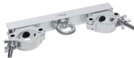
Truss adapter - Ceiling supports CODE S35Tbar Compatibility 32-35mm tube Wide apapter 220mm Tensile load 100 kg Screw plug M10
