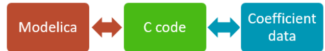
Figure 3. Structure of a thermodynamic property function call in the SBTL model in Modelica.
