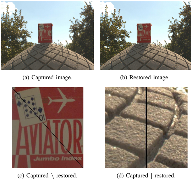
Fig. 15. Example of stray light reduction on a 7 mega-pixel camera image: (a) shows a captured image, (b) shows the restored image, (c) and (d) show a comparison between captured and restored images for two parts of the image.
