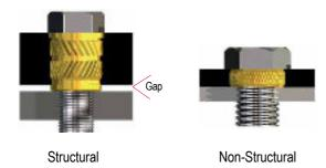
Note: Gap allows for a gasket, (e.g., manifold applications)
