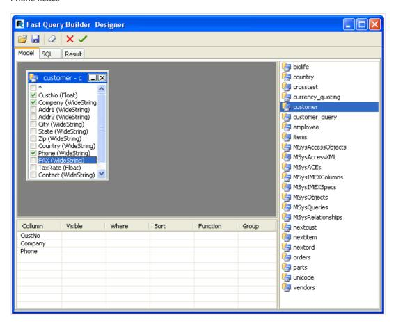
That is all that is required for query building. The query text appears on the SQL tab and the Result tab shows the data returned by the query. Click  $\checkmark$  to close the builder and to return to the query editor, where the query text is now displayed:
