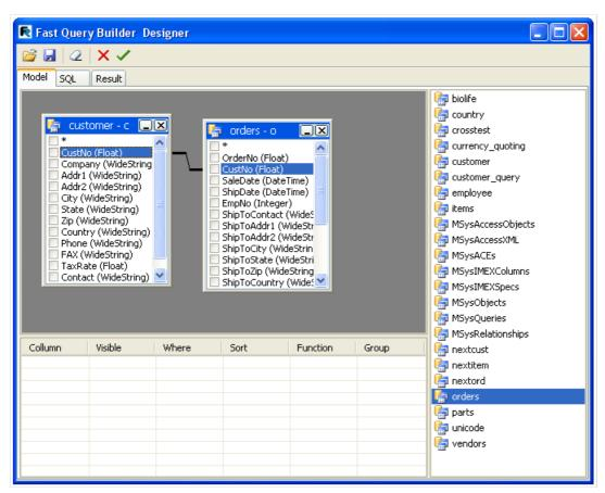
Now the fields to be displayed and the sort field need to be set. Check the "\*" field in both tables and check the CustNo field in the Customer table. The selected fields appear in the field parameters list. Select the sort order for the CustNo field:
