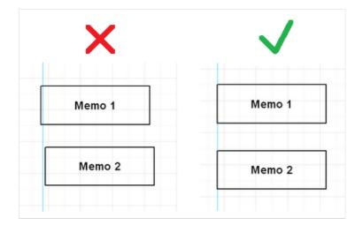
The objects are overlapping - on export to a table/diagram format additional unnecessary rows and columns and also three additional cells in the overlap zone are created:
