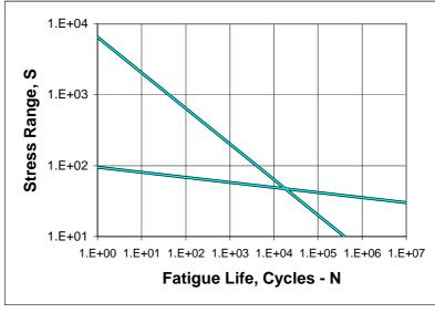
Figure 4: Low-cycle S-N Line (Avakov et al, 1993)
