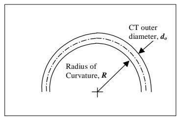
Figure 2: Geometry of coiled tubing when subjected to bending
