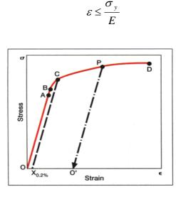
Figure 1: Hooke's law for the stress-strain relationship
