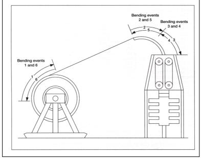
Figure 3: Plastic deformation cycles of coiled tubing during running in and pulling out of a well
