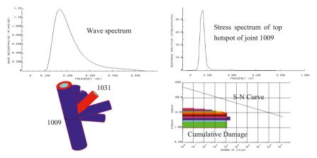
Fig. 6. Stress Spectrum and Fatigue Cumulative Damage Results of joint 1009
