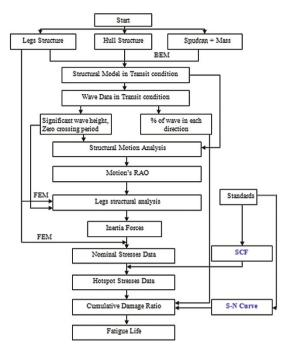
Fig. 2. Fatigue analysis algorithm for jack-up leg structures in transit condition
