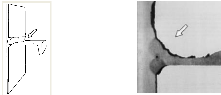
Figure 9.2: Corrosion Necking Effect
