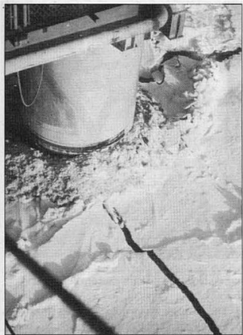
Fig. 3—Ice failure mechanism at a platform leg.
