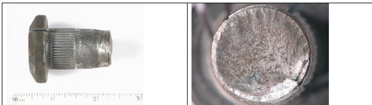
Figure 2: Photographs show one of the broken bolts and its fracture surface.
