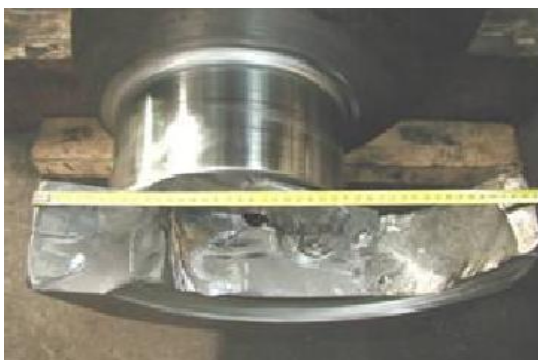
Figure 8.a - Parallel to the axis (final fracture)
