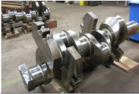
Figure 7 – General view of crankshaft with the fatigue fracture section at junction of n°4 crankpin and forward web
