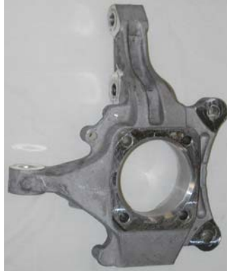
Cast aluminum ASTM A356-T6 steering knuckle of front suspension of a 6-cylinder minivan weighing 2.4 kg
