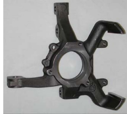
Cast iron ASTM A536 Grade 65-45-12 steering knuckle of front suspension of a 4-cylinder sedan weighing 4.7 kg
