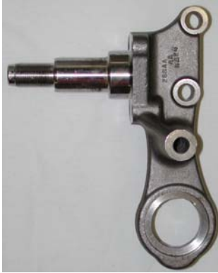
Forged steel SAE Grade 11V37 steering knuckle of rear suspension of a 4-cylinder sedan weighing 2.4 kg
