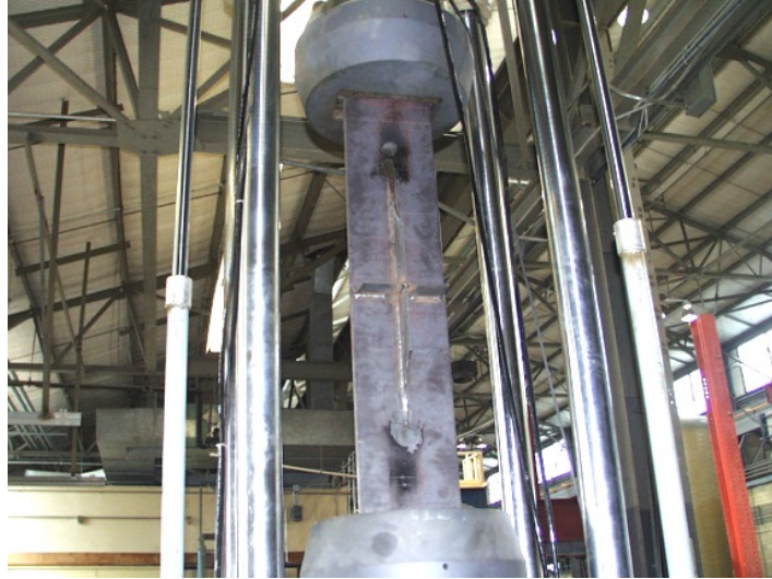
Figure 3-8: Specimen Installed in Test Frame
