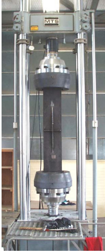
Figure 3-2: MTS Uniaxial Testing Machine with Specimen
