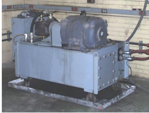
Figure 3-4: MTS Hydraulic Supply Unit
