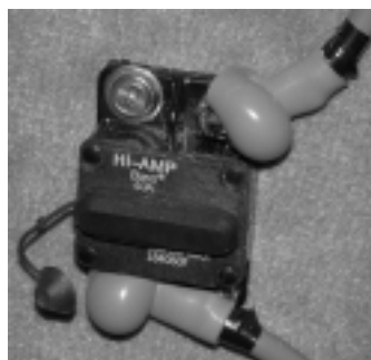
Figure 4-3. Main Circuit Breaker
