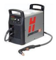
POWERMAX 85 1-1/4" RATED CUT @ 14 IPM 200-600 AUTO VOLTAGE SINGLE OR THREE PHASE W/ BOOST CONDITIONER NEW DURAMAX H85 25' TORCH
