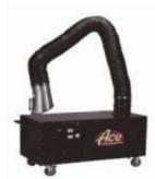
1200 CFM HIGH VOLUME EXTRACTION, DESIGNED FOR SHOP FLOOR WITH MOBILILITY TO MOVE STATIONS. INCLUDES 10' EXTRACTION ARM. HEAVY DUTY STEEL CONSTRUCTION WITH LOCKING CASTERS, BUILT IN AC OUTLET FOR POWER TOOLS
