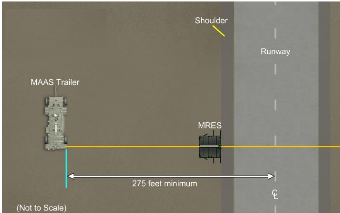
Figure 5-11 Mobile Aircraft Arresting System (MAAS) in Set-Back Configuration with Mobile Runway Edge Sheave (MRES)
