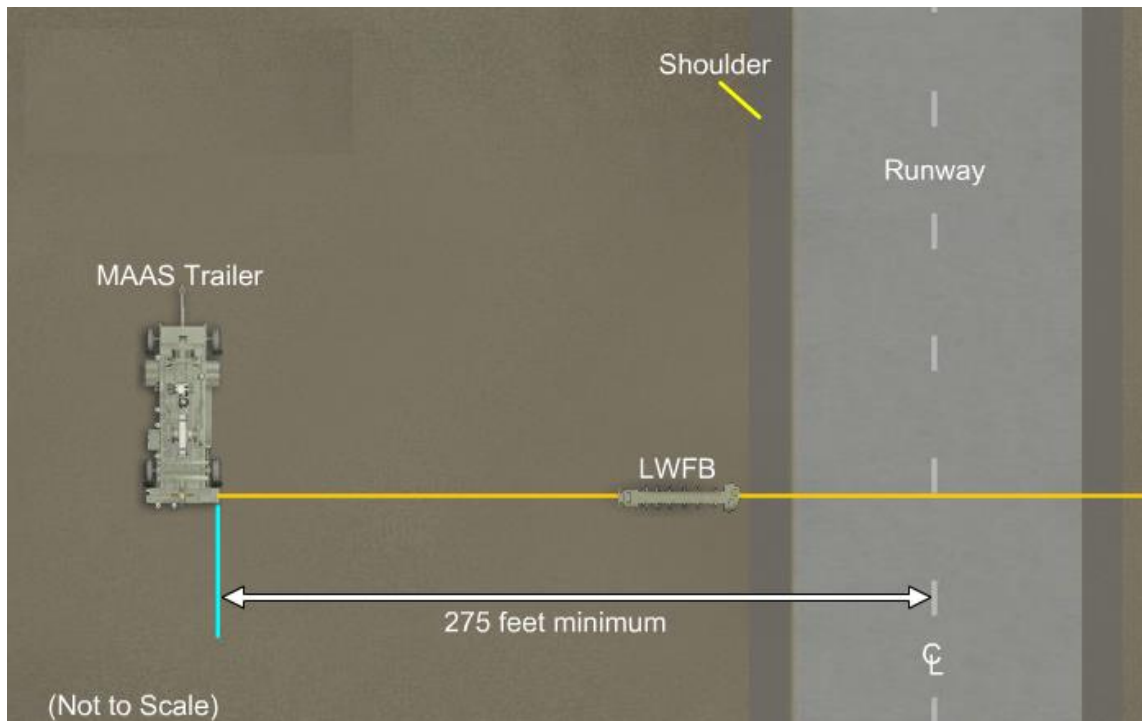
Figure 5-12 Mobile Aircraft Arresting System (MAAS) in Set-Back Configuration with Lightweight Fairlead Beam (LWFB)
