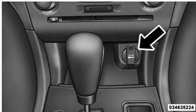
Front Power Outlet
