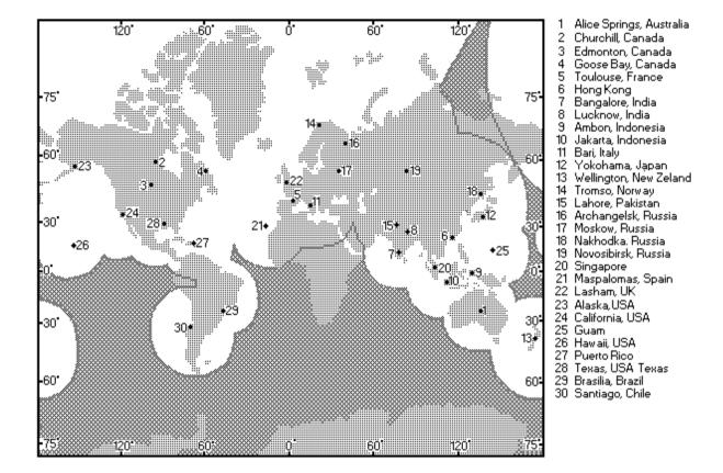
Figure 1b - Satellite Visibility Area of Existing COSPAS - SARSAT LOCAL USER TERMINALS (LUTs)
