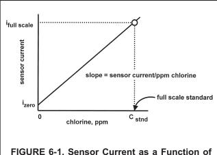
FIGURE 6-1. Sensor Current as a Function of Free Chlorine Concentration
