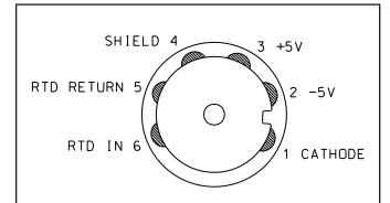
FIGURE 9-1. Pin Out Diagram for Model 498CL-01-VP Sensor (top view of connector end of sensor)
