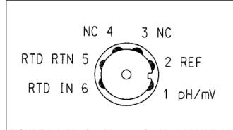
FIGURE 9-2. Pin Out Diagram for Model 399VP-09 Sensor (top view of connector end of sensor)
