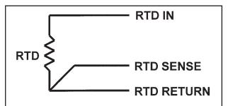
FIGURE 9-4. Three-Wire RTD Configuration.
