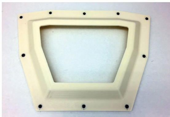
Figure 5. Trim and drill jig printed with ASA.
