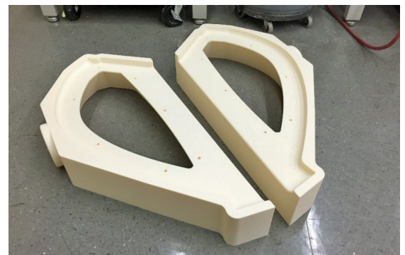
Figure 9. Mirrored halves of the FDM vacuum fixtures upon completion of printing.
