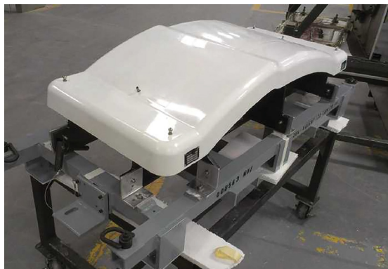
Figure 8. Original machining fixture made out of FRP composites.
