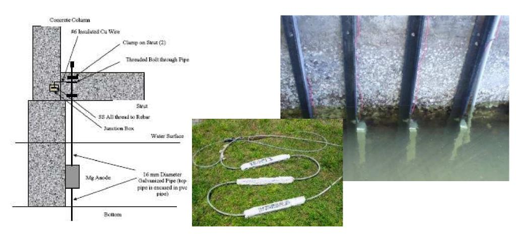
THESE ANODES ARE MOSTLY USED TO PROVIDE CATHODIC PROTECTION TO STRUCTURES WITH UNDERWATER DAMAGE. SIMILAR ARE ALSO USED TO COMPLEMENT GALVANIC PILE JACKETS.
