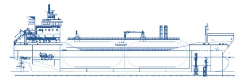
Figure 6.2.1.1 Low pressure, transport volume 6 000  $m^3$ -7 700  $m^3$ , ship length 114 m-150 m.
