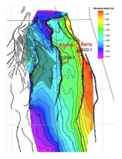
*Figure 7.2.1.1: Smeaheia; the map shows the location of the Alpha and Beta structures in the large fault block located east of Troll.*
