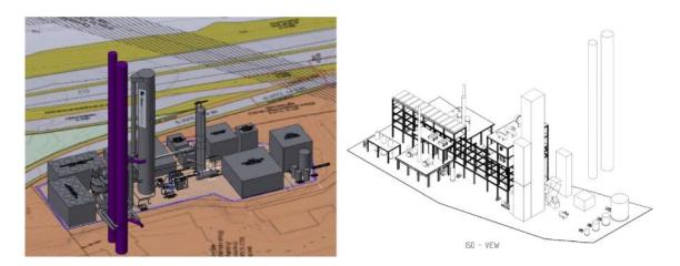
Figure 5.5.1 Sketch of Aker's amine plant (left) and GE's CAP plant (right) at Klemetsrud.
