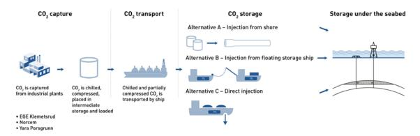
Figure 3.1.1 Schematic presentation of a CCS chain with interfaces.
