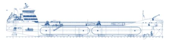
*Figure 6.2.1.2: Medium pressure, 7 400 m<sup>3</sup>–7 770 m<sup>3</sup>, ~160 m.*
