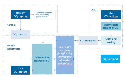
Figure 5.6.1 Joint CO<sub>2</sub> intermediate storage site in Grenland.
