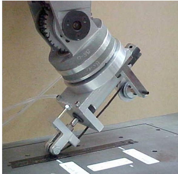
Figure E.1 The roller compaction head mounted on the wrist of the Merlin robot
