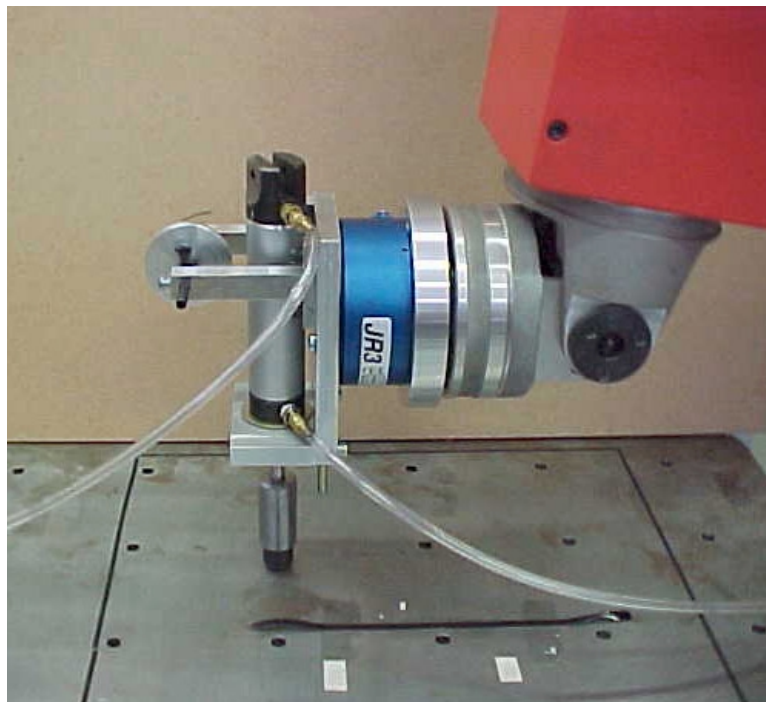
Figure E.2 The ball compaction head mounted on the wrist of the Merlin robot
