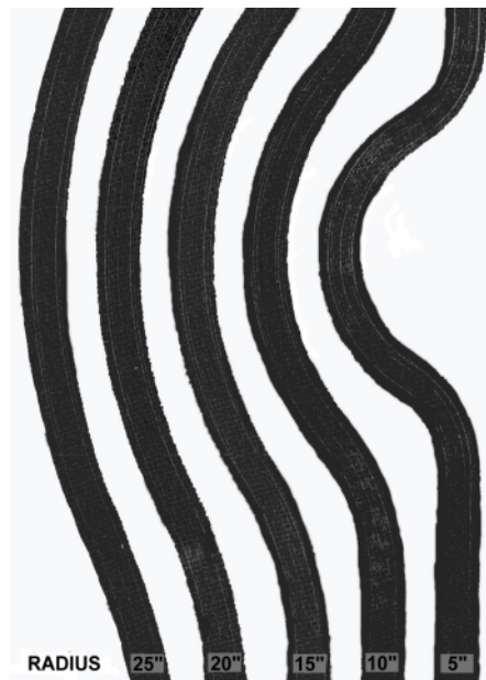
Fig. 1.6 Steered towpreg paths with different radii of curvature [6]
