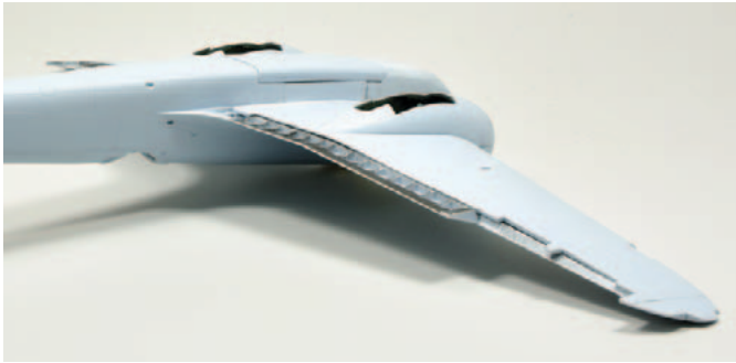
The landing flaps are separate with rib detail moulded into the wings, but it is too heavy...
