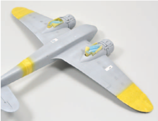
The fuselage band and undersides of the wing tips were painted yellow, then once dry were masked. You can see the other panels, made from plasticard, that were added on the underside
